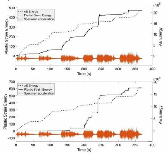
Figure 5. Comparison of accumulated AE energy and accumulated plastic strain energy. BPE (above), BPI (below).
