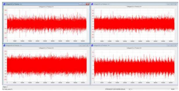
Figure 3: streaming acquisition during 5 sec at 2 Mega sample per second on the four channels.
