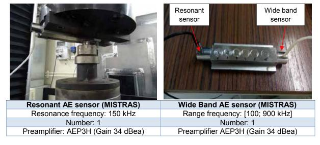
Figure 4. Implementation of the AE sensors on the disc
