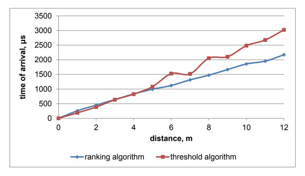
Fig.13. Time of arrival depending on the distance between the source and the sensor
