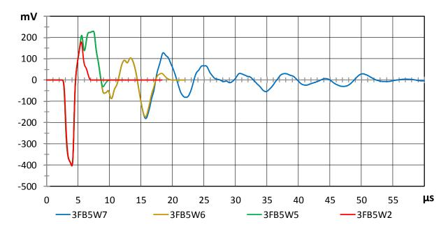
Fig. 2-8 Application of 4 FFT windows (W7, W6, W5, and W2, see last two characters in the legend) on the response of a resonant 150 kHz sensor.
