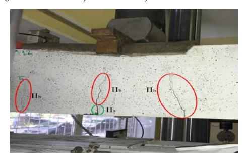
Fig. 7 – The central area of the RC beam M90(2) under the bending test
