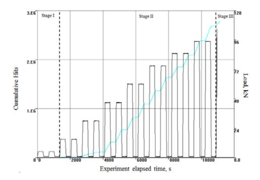
Fig. 5 – Cumulative hits and the load for the RC beam M90(2)
