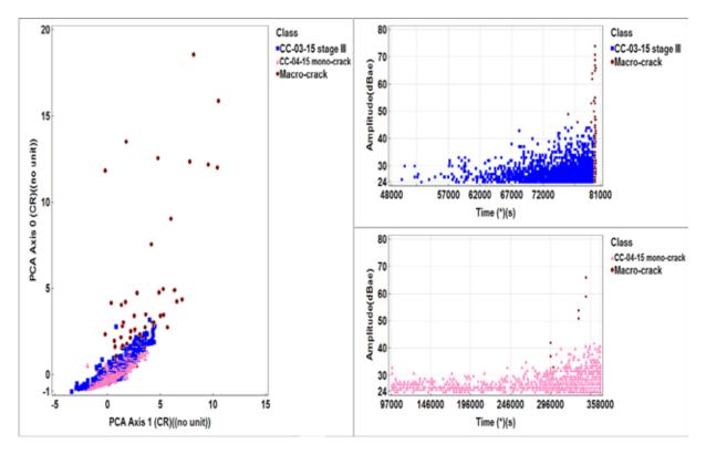
Figure 10: Multiparametric analysis and PCA (Principal Component Analysis) of AE filtered hits recorded during the tests CC-03-15 (multi-cracks) & CC-04-15 (single-crack).
