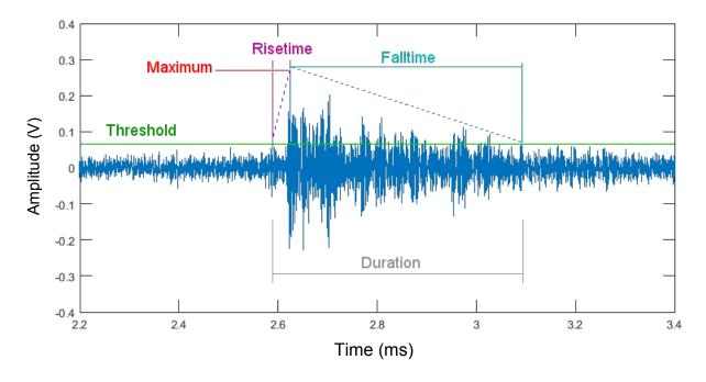
Figure 3. Classical features in AE testing
