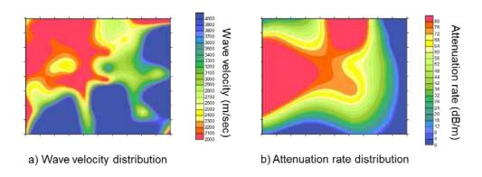
Fig. 7 Numerical analysis for tomography results on wave velocity and attenuation rate
