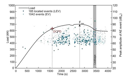
Figure 3. Load and corrected peak amplitudes of all detected AE events (1042 EV and 185 LEV) plotted vs. duration of the bending test of a pipe segment of steel. Highlighted characteristic states in the test progress are the crack initiation determined by DCPD, maximum load of 699 kN and leakage formation.
