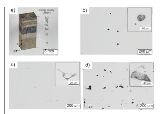
Figure 1: a) Test workpiece produced with three porosity contents; b) — d) Typical light microscope cross-section images of the regions produced with b) 300 mm/s (medium quality), c) 500 mm/s (high quality) and d) 800 mm/s (poor quality).
