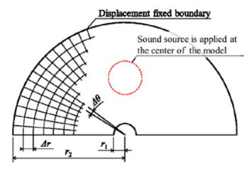
Figure 4 Analysis model of elastic wave in the cylindrical coordinate system [7]
