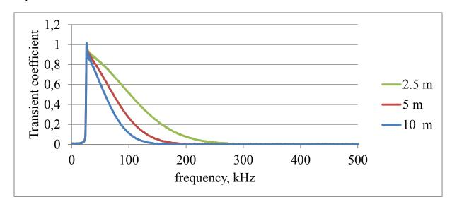
Fig. 10. The transfer function for the attenuation filters
