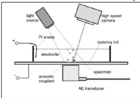
Fig. 2. Schematics of the measurement unit
