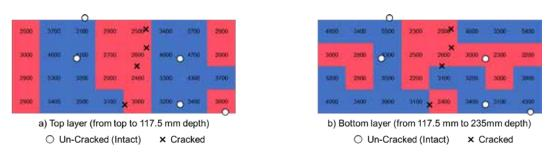
Fig. 9 Wave velocity distribution with quality classification
