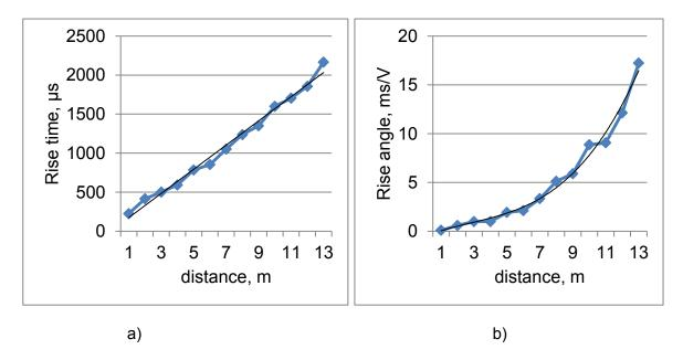
Fig.11 Rise time and rise angle parameters calculated for the modeling signals depending on the distance between the defect and sensor
