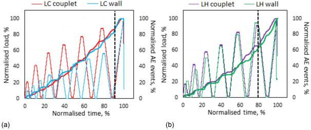
Figure 3. Results of a cyclic test with AE monitoring on a representative sample of (a) lime-cement masonry and (b) lime hydrate masonry.
