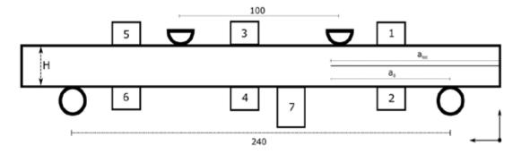
Figure 2: Schematic of the 4-ENF type specimen for mode II (in-plane shear) quasi-static and cyclic fatigue fracture testing of adhesively bonded wood joints, The positions of the AE sensors and the specimens dimensions are also shown (H = 10 mm,  $a_{tot} = 110 \text{ mm}$ ,  $a_0$  approximately 70 mm).
