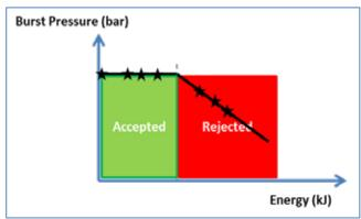
Figure 6: Burst pressure reduction curve, with respect to impact energy.
