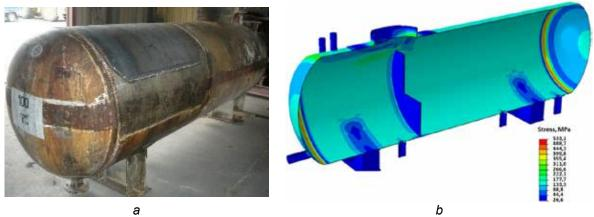
Fig. 5. The pressure vessel (a) and von Mises stress distribution in the shell under 1,0 MPa pressure (b)
