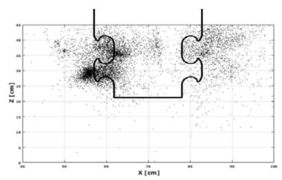
Fig. 7: Position of the located events in a projection onto the x-z-plane together with the contour of the concrete dowel in an enlarged view.
