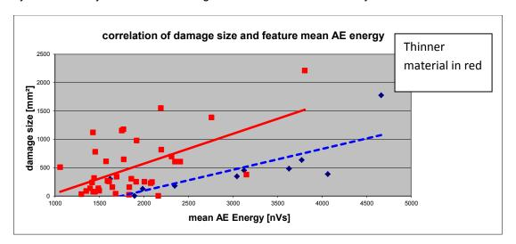
Figure 13: Correlation of damage size and acoustic mean energy (AE signal) delivered by the AE
