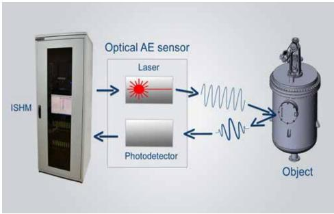
Fig. 6. Simplified scheme of the optical AE sensor at the AE ISHM system
