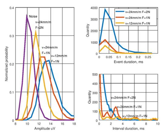
Figure 2 – Distributions of AE features during scratch test of a copper polycrystal. Amplitude distribution (left); Signal duration distribution (top right); Inter-arrival interval distribution (bottom right)
