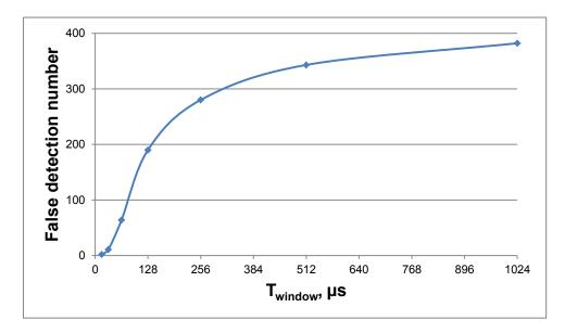
Fig.5 The number of false impulse detections depending on the duration of time interval
