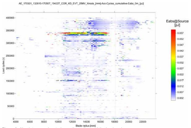
Figure 8: Absolut energy located over the radius and the load cycles
