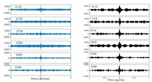
Fig. 8: Cross-correlations (CCF) of all TR signal pairs detected at the source point.
