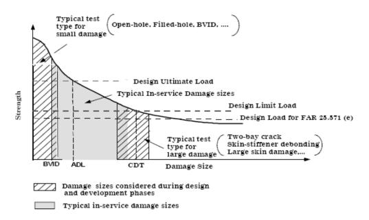
Figure 2: Residual Strength versus damage size Relationship [4]
