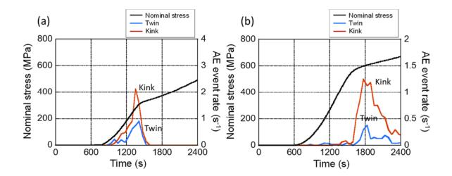
Fig. 4 AE event rate of twinning and kinking in (a) Mg<sub>97</sub>Zn<sub>1</sub>Y<sub>2</sub> and (b) Mg<sub>89</sub>Zn<sub>4</sub>Y<sub>7</sub>.
