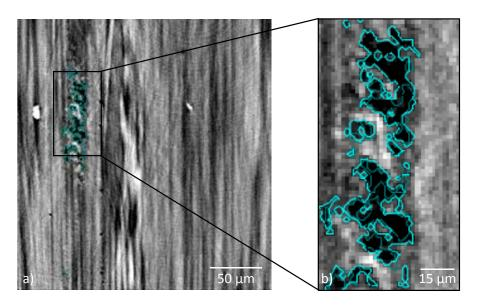
**Figure 3.** a) Crack evolution as identified on a single slice of the highest strains scanned volume b) zoomed region showing in black the crack at the highest strains with its contours in light cyan. In darker cyan, the contours of the same less developed crack as detected with the growth segmentation tool in a scanned volume at lower strains.
