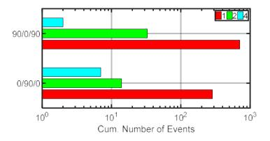
Figure 3: Cumulative number of events in the classes 1, 2 and 4 for the 90/0/90 and 0/90/0 specimen
