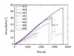
Fig. 3. Stress versus time for all the tested beams. Red: Non-reinforced beams (NR). Blue: Longitudinal reinforced beams (LR). Black: Braided reinforced beams (BR).
