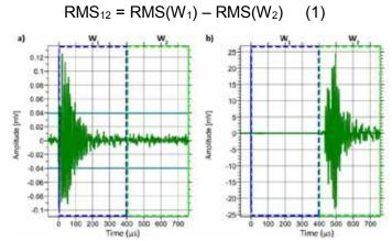
Fig. 5. Example of two AE signals. a: Well recorded signal. b: Mis-recorded signal.
