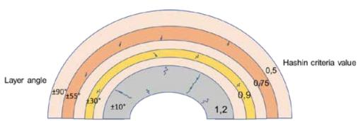
Figure 11: Overview of accumulator layers with Hashin criteria evaluation for a proof test pressure of 300 bar
