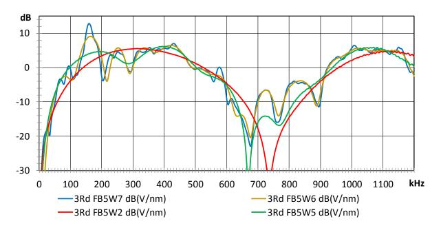
Fig. 2-9: Displacement receiving sensitivities derived from the time-series signals in Fig. 2-8.
