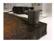
Figure 1 - Sensor F-15α on steel surface. Coupling is insured with silicon grease.
