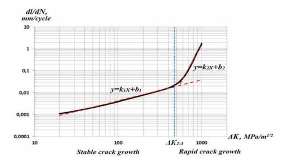
Fig. 4 Typical KDFF, registered during experiment: **dl/dN** – the crack length *l* change during **N** loading cycles; **ΔK** – stress intensity factor peak-to-peak range
