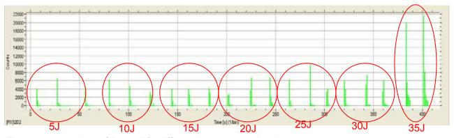
Figure 15: comparison of "counts" for different impact energy levels
