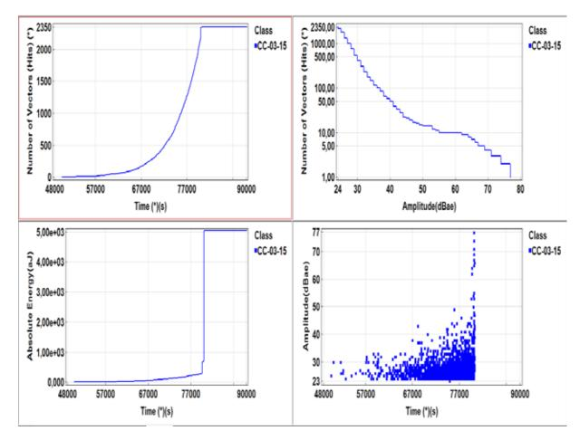
Figure 7: Filtered AE results recorded during the following tests (Stage III [t>48000 s]: CC-03-15), Plot 1: Cumulated Activity of AE hits as a function of time, Plot 2: Cumulated Intensity of AE hits as a function of time, Plot 3: AE hits number as a function of their amplitude, Plot 4: AE hits amplitude as a function of time.
