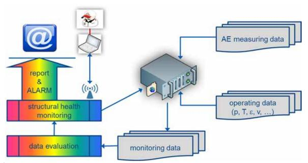
Figure 1: Acoustic emission monitoring concept
