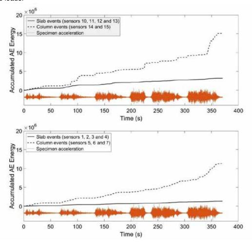
Figure 3. Accumulated AE energy at column-slab connections. AbE (above), AbI (below).
