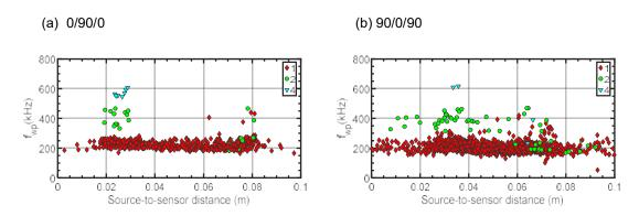
Figure 7: Change in Weighted peak frequency as a function of source-to-sensor distance for specimen 0/90/0 (left side) and 90/0/90 (right side). The colors represent the classes
