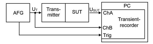
Fig. 2-1 Block diagram of face-to-face setup
