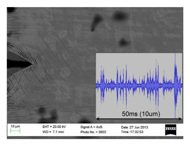
Figure 3 - Comparison between the surface topology in front of the indenter tip and the AE signal after noise reduction.
