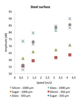
Figure 4 - Amplitude as function of particle's speed for steel surface.
