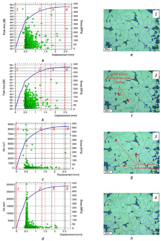
Fig. 4. Stress-strain curves of B type specimen with AE signal amplitude (a, b) and RA parameter distributions (c, d) for VS150-M type sensors (a, c) and VS75-V type sensors (c, d) as well as material microstructure images (e ÷ h) for different stress levels, magnification 600×
