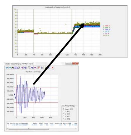
Figure 2: acquisition with smart threshold (above graph) and waveform and hit correspondence (graph below).
