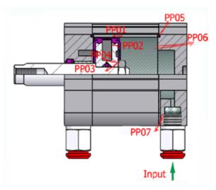
Figure 4. Leaks below the piston during progress stroke [11]
