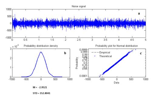
Figure 4. The steady process, whose amplitudes are normally distributed within the single waveform indicates the absence of agglomerates.
