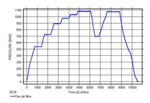
Figure 3: Pressure sequence for 36L vessels.
