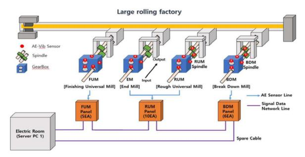
Fig. 3. Schematic diagram of large rolling factory gear box health monitoring system
