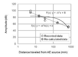
Fig. 2 Linear estimation on travel time amplitude from AE source to sensors
