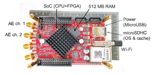
Figure 2. Photo of the wireless sensor node (STEMlab125-14 board)
