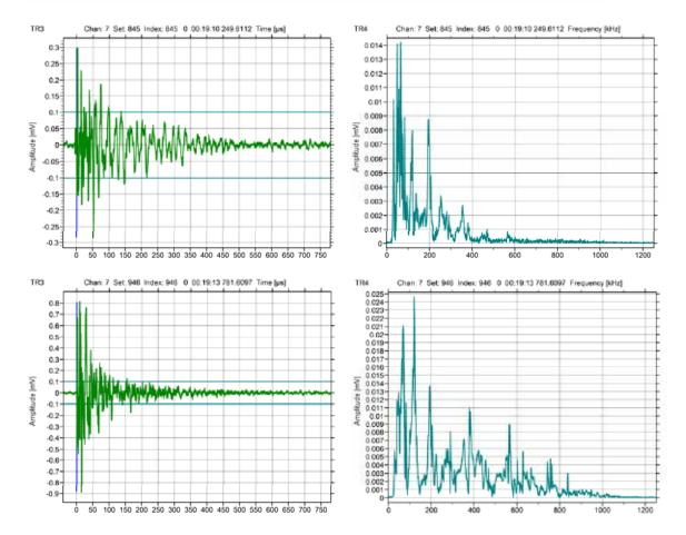
Figure 11: Selected AE waveforms and Fast Fourier Transform power spectra for one PRF adhesive joint from the broad-band AE sensor mounted in the propagation zone of the delamination.
