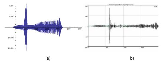
Fig. 6. a) Model signal for thickness of 17 mm and a distance of 5 m, created on the basis of the Morlet wavelet with a center frequency of 160 kHz; b) the actual signal received by the GT200 sensor on the 17 mm plate at a distance of 5 m from the source
