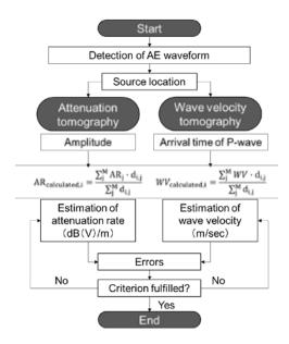
Fig.1 Flow chart to compute wave-velocity and attenuation-rate tomography
