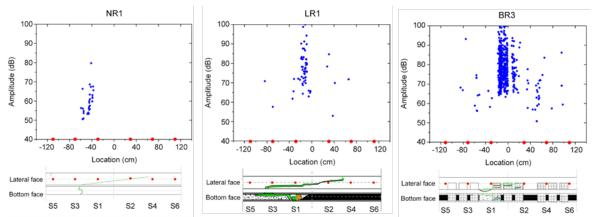
Fig. 5. AE linear location of events (Group 2) during the bending test for an example of non-reinforced (NR), longitudinal reinforced (LR) and braided reinforced (BR) beam.
