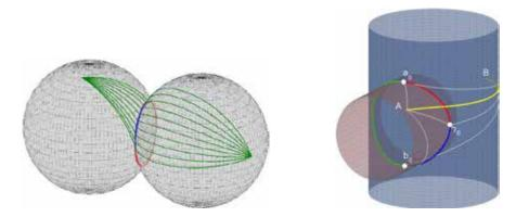
Figure 1: Computing geodesics through intersection on compound body.
