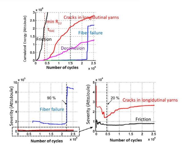
Figure 6 : Evolution of the activity of several damage mechanisms during the loading phase of a cyclic fatigue test.
