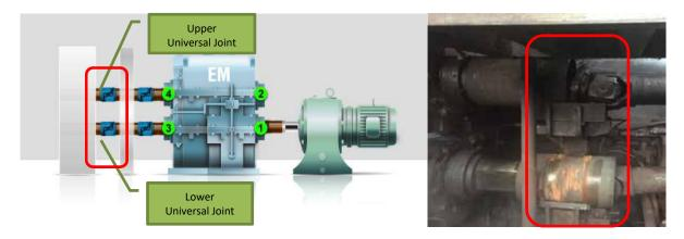
Fig. 5. EM Gear box Universi Joint breakage position (left) and damage picture (right)
