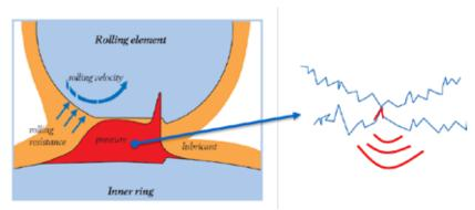
Figure 1: AE signal from asperity in rolling contact
