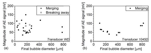
Fig. 4. Amplitude of the acoustic signals and the final size of the merged bubbles: (a) transducer WD by PAC; (b) transducer 1045 by Fujicera.
