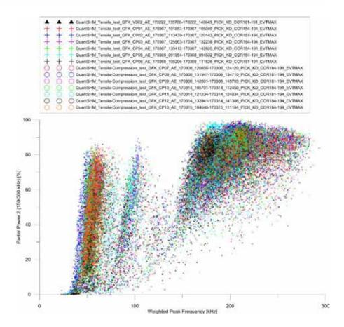
Figure 4: Partial power of the burst signals against their the weighted peak frequency (WPF)[3]
