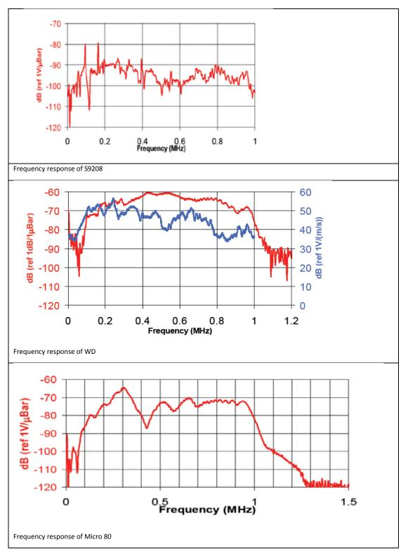
Figure 4: calibration curves of sensors \$9203, WD and micro 80.
