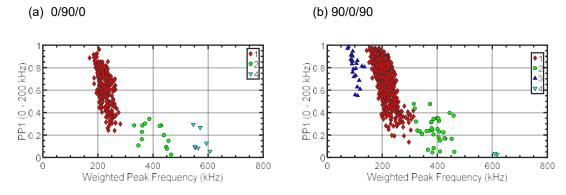
Figure 2: Signal classification through AE Features Partial Power 1 (-) and Weighted peak frequency (kHz) of 1<sup>st</sup> Hit of events for specimen 0/90/0 (a) and 90/0/90 (b) with color coded classes
