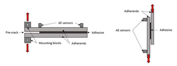
Figure 1. Double Cantilever Beam experimental schematic (not to scale)
