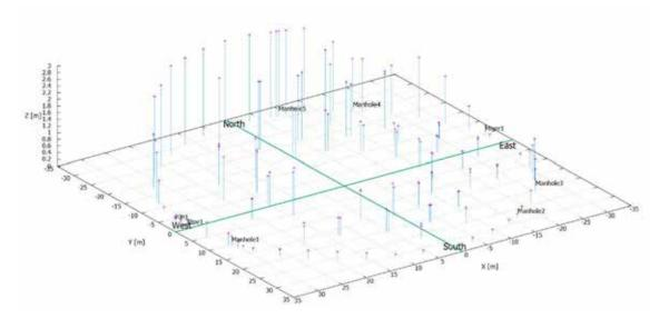
Fig 5. Spatial visualization of the sludge heights at the measurement points on the bottom of the tank
