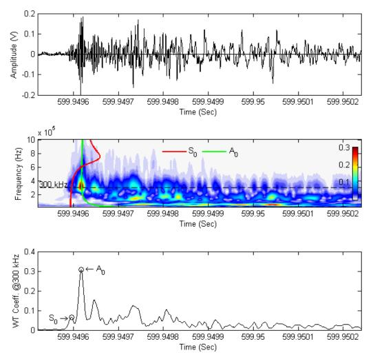
Figure 3. Example of signal-processing method. Top: Original AE signal. Middle: Wavelet Transform plot with overlaid dispersion curves indicating symmetric (S0) and asymmetric (A0) wave-modes. Bottom: Wavelet Transform coefficients for 300 kHz frequency band, with  $S_0$  and  $A_0$  peaks marked.
