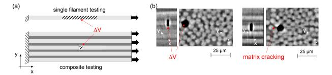
**Figure 3.** Schematic difference in  $\Delta V$  for single filament testing vs. fibres confined within composite material (a) and experimental measurement of  $\Delta V$  using high-resolution computed tomography at 0.4  $\mu$ m voxel size (b).
