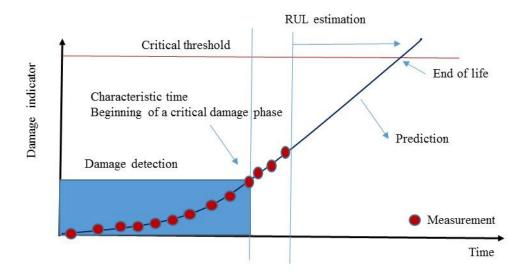
Figure 1: Prediction of lifetime of Ceramic Matrix Composite during long-term mechanical tests
