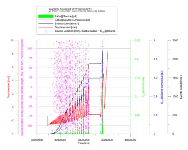
Figure 3: Results for the Probe CP01 - Displacement (red), Source location (magenta) [3]
