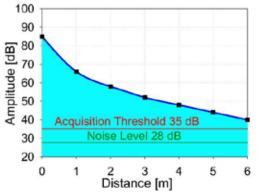
Figure 3. Experimental curve of acoustic waves damping out
