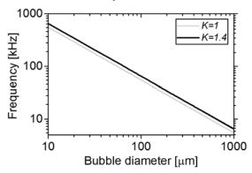
Fig. 1. Resonance frequencies of the hydrogen bubbles according to Eq.(1)
