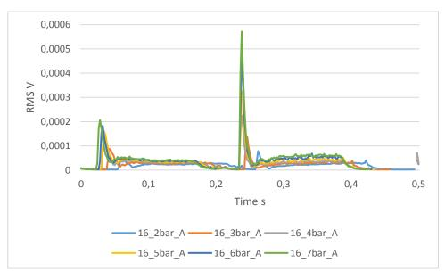
Figure 11. Influence of air pressure on the form of AE signal
