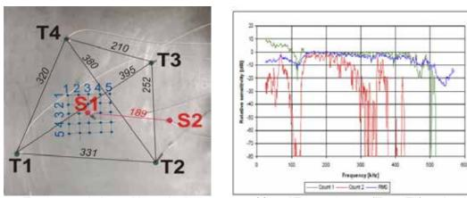
Fig. 1: Testing steel plate with marked placement of four AE transducers (T1 to T4) and artificial AE sources (S1, S2) – left. Right is frequency response of the IDK 09 transducers.
