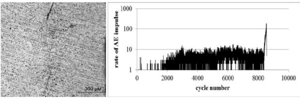
Fig. 8 a. Metallographic image of the additional fatigue crack b. increasing of AE activity vs cycle number due to the presence of additional defects
