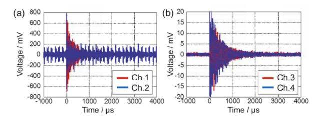
Figure 4. Typical waveform of an AE event recorded by (a) wired and (b) wireless CWM
