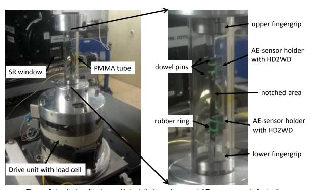
Figure 2. In situ tensile stage with installed specimen and AE sensors ready for testing.
