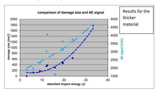
Figure 11: Comparison of damage size and AE signal over the absorbed impact energy for the thicker panel
