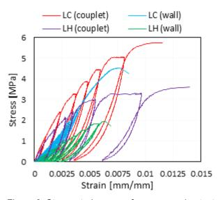
Figure 2. Stress-strain curves for compression tests on masonry couplets and walls.
