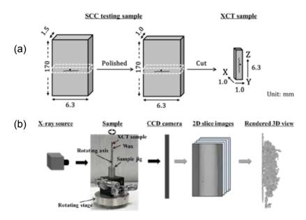
Fig. 2 (a) Schematic of the preparation of XCT sample, (b) 3D X-ray computed tomographic process of internal view of cracks.
