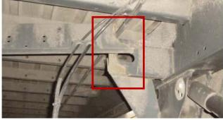
Figure 1. Damages to semitrailers at junction plate (left) and transverse beam (right)
