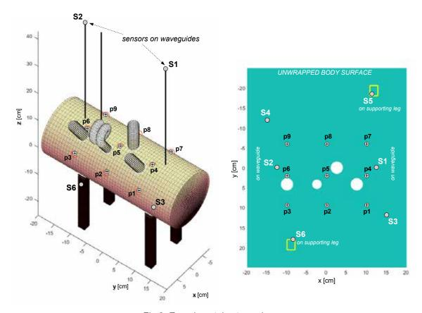
Fig.3: Experimental setup scheme.
