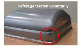
**Figure 4.a.** part with a real defect caused by the tool. b. part with a defect generated voluntarily by correcting the punch
