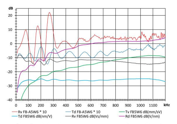
Fig. 3-5 Transmitting and receiving sensitivites using transmitter B and deviation to A
