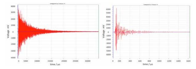
Figure 7 - Waveforms for steel surface (left) and plastic surface (right). Silicon particles were used and their speed was fixed to 3,13 m/s. The different attenuation of the signal could be easily observed.
