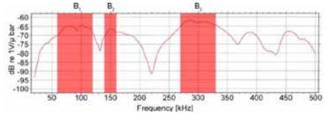
Fig. 3. Sensitivity curve of the multi-resonant sensor VS45-H.
