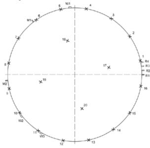
Fig 3. An example of the layout of AE sensors on the tested storage tank
