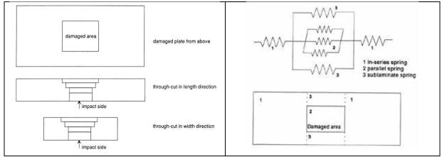
Figure 16: a) Idealization of the characteristic state of damage after impact. b) Areas representing springs in one-dimensional spring model (source: Fraunhofer LBF)
