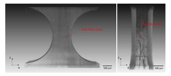
**Figure 4.** Frontal (left) and lateral (right) view of the region of interest, kept the same for all the scanned volumes. The inter-fibre crack is shown in red as identified in the highest strains scans. The combined use of a visual approach and an automated growth segmentation tool on VGStudio MAX<sup>TM</sup> allowed the user to identify the crack evolution from lower to higher strains.
