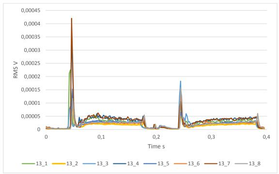
Figure 8. Effect of sensor positioning on signal form
