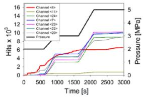
Figure 4. Fragment of reactor loading during hydrotesting and AE in the Total Hits – Time coordinates on all AE registration channels
