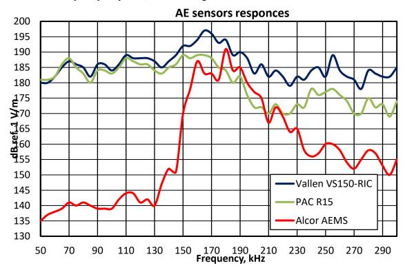
Fig. 5. Frequency responses of the AEMS (red) and industry standard resonant sensors.
