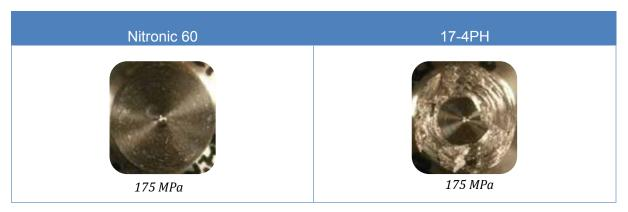
**Table 2.** Tow types of galling are generated on Nitronic60 and 17-4PH under the same load 175MPa (tolerant galling, catastrophic galling)
