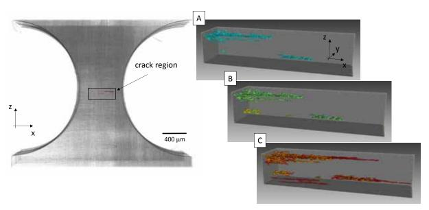
**Figure 5.** Visualization of inter-fibre crack and volumetric evaluation at three load levels (A-C) as noted in Figure 6.
