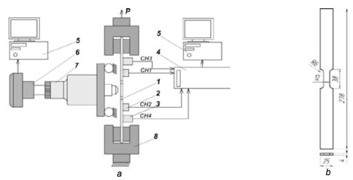
Fig. 2. Diagram of the testing station (a) and technical drawing of tested specimen (b): 1 – specimen, 2 – VS150-M type sensors, 3 – VS75-V type sensors, 4 – AE measurement system, 5 – computers, 6 – digital camera, 7 – light portable microscope, 8 – testing machine's grips
