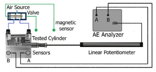
Figure 1. Scheme of the measuring chain
