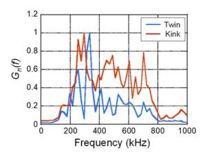
Fig. 3 Normalized average energy spectra of twin and kind for learning data.
