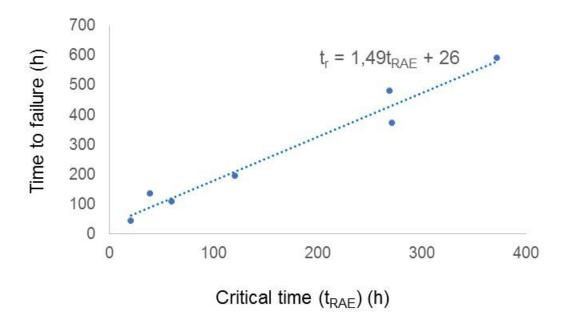
Figure 7 : Correlation between the characteristic time  $t_{\text{RAE}}$ , obtained with the minimum of the coefficient of emission, and the experimental time to failure.
