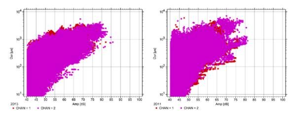
Figure 9: AE signal parameter plots (duration versus amplitude) of quasi-static tests using the AE sensors located near the starter crack tip of the 4-ENF specimens with (left) PRF and (right) HB110 adhesive (following [6]).
