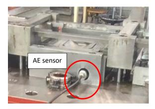
Figure 5. Implantation of AE sensor close to the stamped parts
