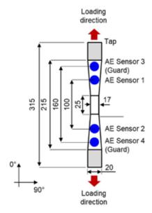
Figure 1: Specimen dimensions and experimental setup for the quasi-static tensile testing of CFRP coupons
