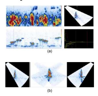
Figure 3 – (a) Step-wise damage (b) Through-thickness damage indication
