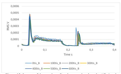
Figure 13. Impact of the number of cycles completed on the AE signal
