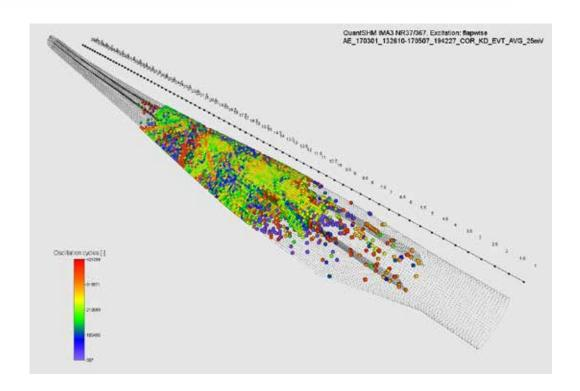
Figure 6: Overall view of the rotor blade with the cumulated event distribution depending on the load cycles (purple: early, red: late during the experiment)
