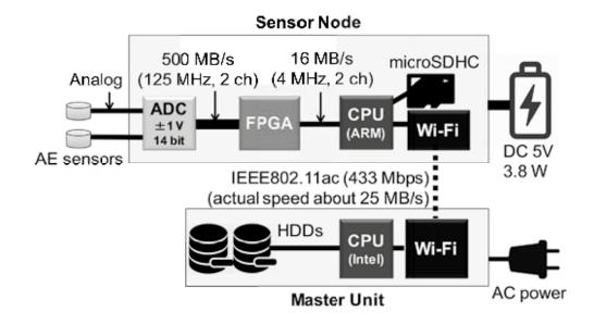
Figure 1. Schematic diagram of the data flow of the wireless CWM system
