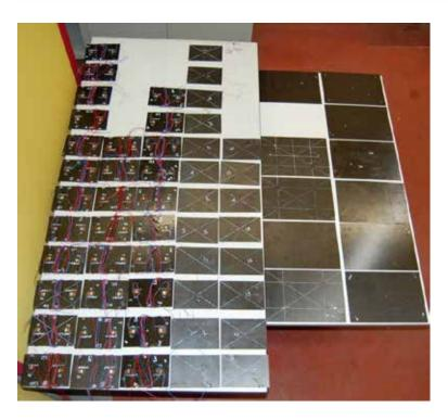
Figure 5: Overview of the panels for CAI (left) and the original size for Impact tests (right)
