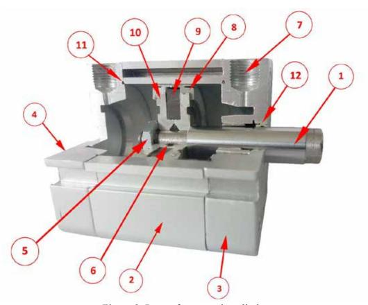
Figure 2. Parts of pneumatic cylinder
