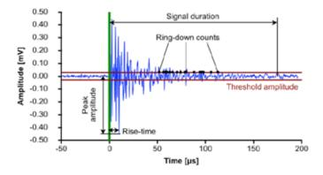
Fig. 4. Typical AE burst signal. Peak amplitude, signal duration, signal rise-time and ring-down counts are indicated. The threshold amplitude corresponds to 30 dB.
