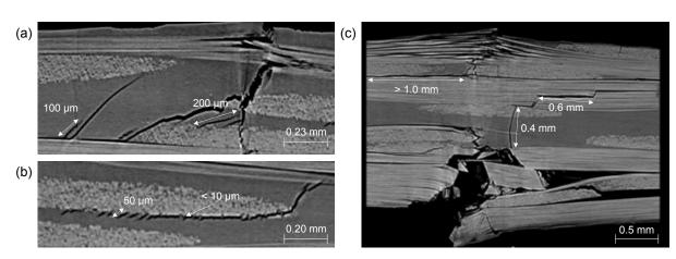
**Figure 2.** Computed tomography image of crack network on microscale (a and b) and on macroscale (c) taken from damage region of four-point bending sample of [10], [12].
