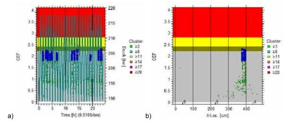
**Figure 7:** Evaluation of passivation air cylinder a) CEF and pressure vs. time, b) CEF vs. X-Location.
