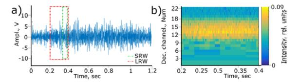
Figure 2: a) A typical AE signal from one complete layer of medium quality (300 mm/s). The red and green boxes are the long (LRW) and Short Running Windows (SRW) scanning the acquired signal; b) reconstructed spectrogram for the LRW time span bounded by red lines in Fig. 2, a).
