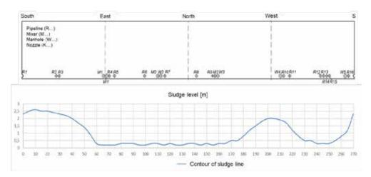
Fig 2. The line contour of sludge along circumference tank wall
