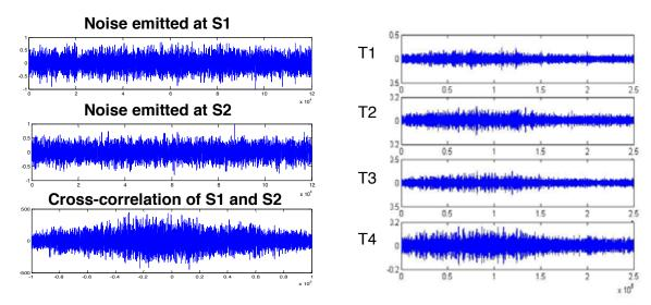
Fig. 10: Left – noises emitted at S1 and S2, and their cross-correlation. Right – mixed signals recorded by transducers T1 to T4.
