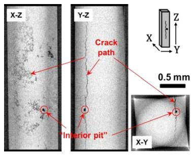
**Fig. 5** Reconstructed tomographic slices showing an "interior pit" along the crack path of the sample C. The inserted schematic indicates the planes.
