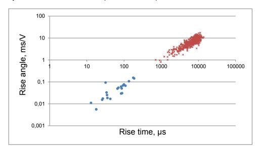
Fig.4. Scatterplot Rise angle vs Rise time for AE signal (blue points) and friction noise (red points)
