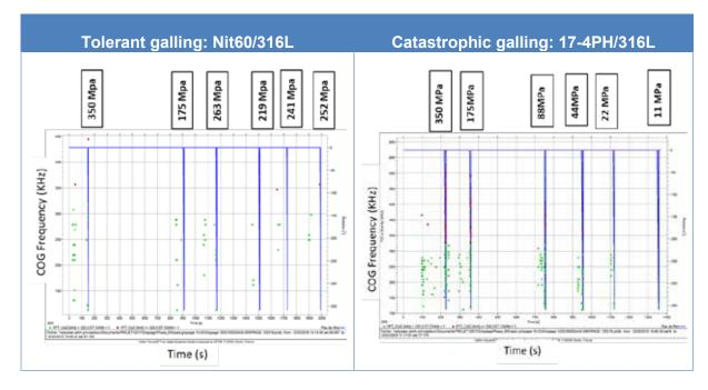
**Figure 8.** Comparison between tolerant galling and catastrophic one "distribution of the centroid frequency as function of the time test under different loads (green points represent frequency <320 KHz; red ones represent frequency >320 KHz)
