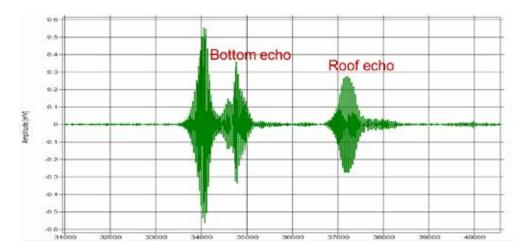
Fig 4. The wave propagation and wave reflection in storage product between AE sensors
