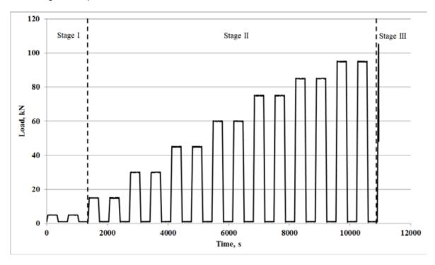
Fig. 3 – Loading scheme for RC beam M90(2)
