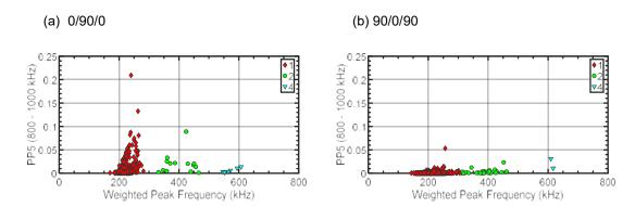
Figure 5: Partial Power 5 (-) and Weighted peak frequency (kHz) of 1st Hit of events for specimen 0/90/0 (a) and 90/0/90 (b) with color coded classes
