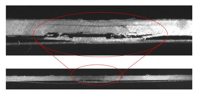
Figure 8: Microscopic analysis of delaminations.
