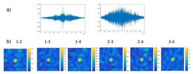
Fig. 18: a) Cross-correlations of 2 TR reconstructions at the source (left) and at the plate corner (right), b) Distributions of CCFs maxima at 30x30 mm region around the source.
