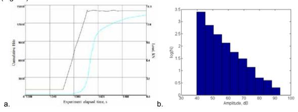
Fig. 8 – (a) Cumulative hits and the load for the RC beam, (b) Amplitude distribution for loading to 15 kN (first loading cycle of the second loading step)
