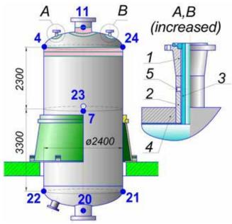
Figure 2. Hydrotreating reactor arrangement: ● 11/ ○ 23 - location of AE transducers and channel number from the visible / back side, 1 – nozzle flange, 2 – nozzle neck, 3 – nozzle sleeve, 4 – bimetal vessel bottom, 5 – test hole, □ - area of ultrasonic testing
