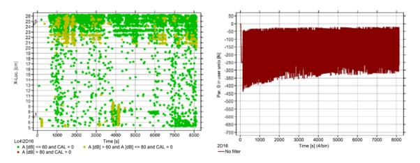
Figure 8: (left) AE linear signal source location (color-coded for AE signal amplitude) of dynamic 4-ENF tests at 5 Hz using the AE sensors on the compression side and (right) load curve for the 4-ENF specimen with the HB110 adhesive.
