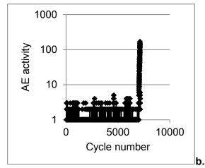
Fig. 5 Dependence of cumulative hit counts and AE activity vs. loading cycle number
