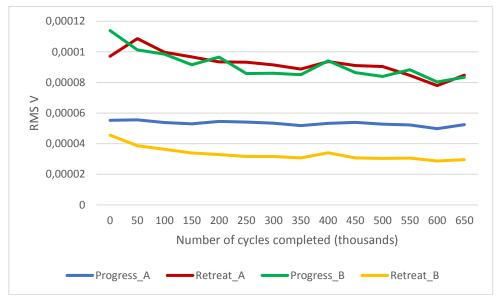
Figure 14. Impact of the number of cycles completed on the average value of RMS when sliding and inserting
