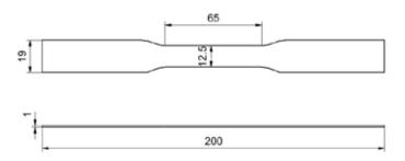
Fig. 1. Dimensions of the tensile specimens in mm.
