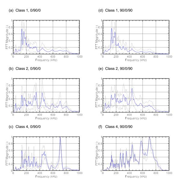
Figure 4: Standardized and averaged Fourier transforms of acoustic emission signals (blue line) from classes 1, 2 and 4 from specimen 0/90/0 (a,b,c) and 90/0/90 (d,e,f) along with their standard deviation (black dotted line)
