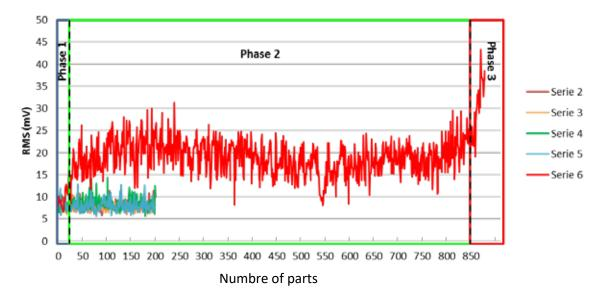
Figure 11. Evolution of the RMS (mV) as function of the number of stamped parts
