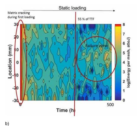
Figure 2 : a) Evolution of the coefficient R<sub>AE</sub> and b) Location of the acoustic emission signals and the recorded energy versus time for a static fatigue test at 500 °C and  $\sigma_{applied}/\sigma_r$ =0.44, the colour scale represents the recorded energy in a mesh.
