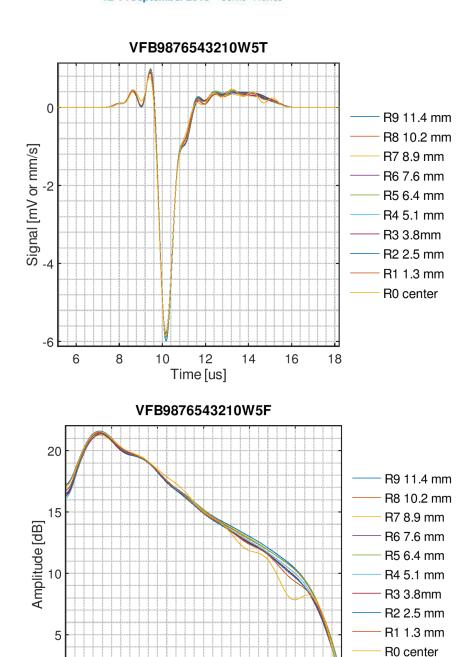
Fig 3-3 like Fig. 3-2 but window size shortened from W6 to W5.
