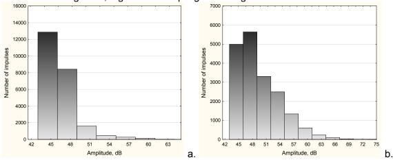
Fig.6 Histograms of amplitudes distribution at different stages of fatigue crack growth a. for stable stage b. for accelerated growth
