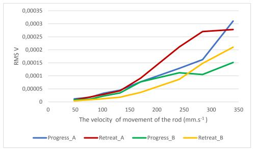
Figure 10. Effect of piston movement velocity on the average value of RMS when sliding and inserting
