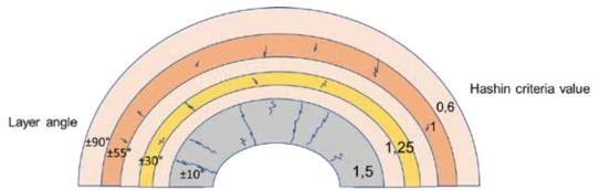
Figure 12: Overview of accumulator layers with Hashin criteria evaluation for a proof test pressure of 450 bar
