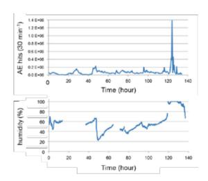
Fig. 4 AE activities and relative humidity during measurement
