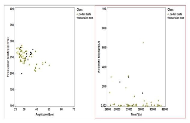
Figure 8: Frequency centroid of AE hits as function of their amplitude; Absolute energy of AE hits versus time (Stage II [24000 s - 48000 s]: Loaded tests CC-02-15, CC-03-15 & CC-07-15 – Immersion test CI-01-15).
