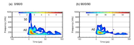
Figure 8: Continuous wavelet transforms of exemplary signals of class 1 from specimen 0/90/0 (left side) and 90/0/90 (right side)
