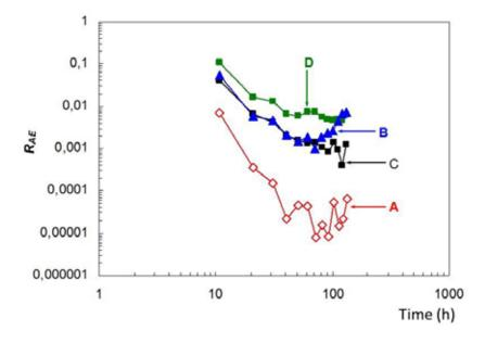
Figure 5: Evolution of the RAE coefficient for the four clusters identified during static fatigue test
