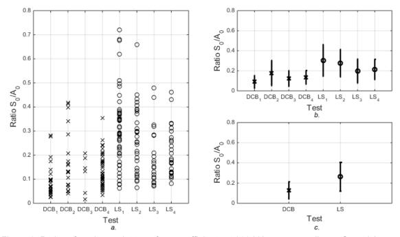
Figure 6. Ratios of peak wavelet-transform coefficients at 300 kHz corresponding to  $S_0$  and  $A_0$  wavemodes. (a) All hits analysed. (b) Mean and std. deviation for each test. (c) Overall mean and std. deviation for the two test types.
