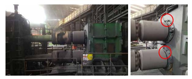
Fig. 4. Installation of AE-Vib. Sensor around large rolling factory
