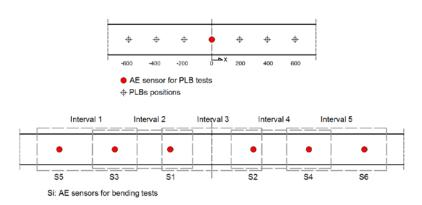
Fig 2. Attenuation tests procedure
