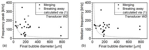
Fig. 5. (a) frequency peak and (b) median frequency of the signals collected by the transducer PAC WD.
