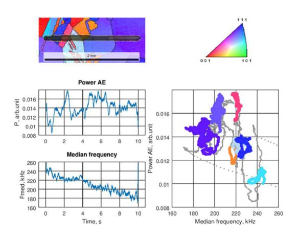
Figure 4 - Power and Median Frequency of Acoustic Emission for a Scratch Test (Copper, 12 mm / min, 1N)
