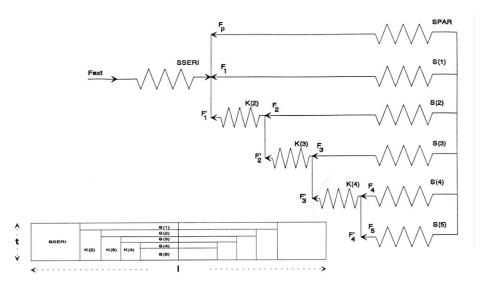
Figure 18: Spring Model (one half of the plate) (source: Fraunhofer LBF)
