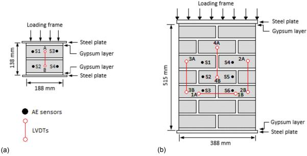
Figure 1. Test setup for compression test on masonry (a) couplet and (b) wall.
