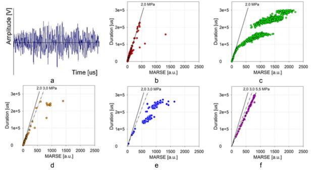
Figure 7. Typical shape of AE signal from product leakage via the through hole (a) and AE signal distribution registered on Channel 4 in Duration-MARSE coordinates during 2.0 MPa pressure hold (b), 3.0 MPa (d), 5.0 MPa (f), and during pressure buildup (loading) from 2 to 3 MPa (c) and from 3 to 5 MPa (e)
