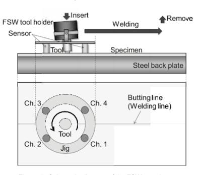
Figure 3. Schematic diagram of the FSW experiment
