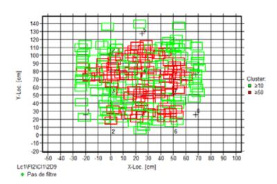
Figure 5: Cluster localization of a healthy vessel after 100 cycles at 875 bar.
