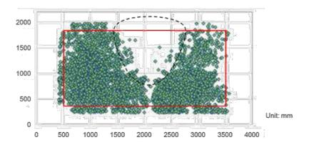
Fig. 5 Result of AE source location analysis
