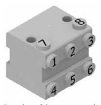
Figure 7. Location of the sensors on the cylinder
