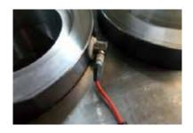
Figure 10. Implantation of AE sensor close to the stamped parts
