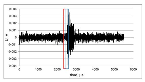
Fig.1. AE impulse against background noise, two time intervals are marked with color rectangles
