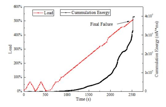
Fig. 2 The cumulative energy by No. 8 sensor during Loading process
