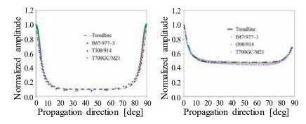
Figure 2 Relationship between normalized amplitude and propagation direction of Lamb wave AE in cross-ply CFRP generated with dipole source. (Left: Fd=0.64 for  $S_0$ -mode,Right: Fd =0.32 for  $A_0$ -mode)[3]
