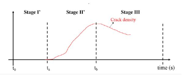
Figure 3: Representation of the different times and stages of crack colony evolution according to DIC & EN measurements [24]
