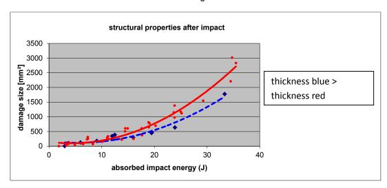
Figure 9: Damage Size over absorbed impact energy
