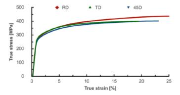
Fig. 2. True stress-strain curves of commercially pure titanium at room temperature parallel to the rolling direction (RD), transversal direction (TD) and under an angle of 45° with the rolling direction (45D).
