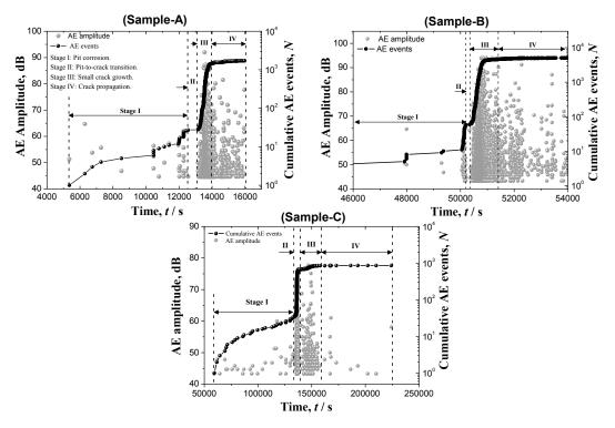
**Fig. 6** Evolution of cumulative events and amplitude of AE signals obtained during SCC evolution of samples A, B, and C.
