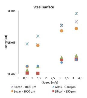
Figure 3- Energy as function of particle's speed for steel surface
