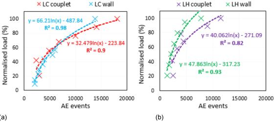
Figure 5. Normalised load vs. number of AE events for (a) lime-cement masonry and (b) lime hydrate masonry.
