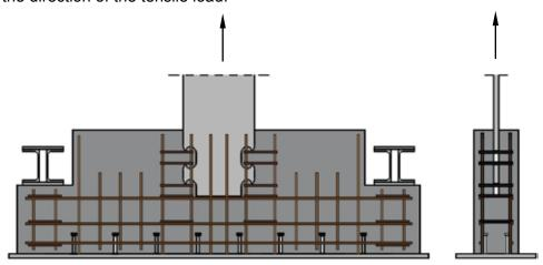
Fig. 1: Front view (left) and side view (right) of the specimen of reinforced concrete with position of the embedded steel anchor with a clothoid-shaped form and the vertical and horizontal reinforcing bars. The arrows indicate the direction of the tensile load.
