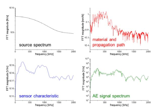
**Figure 5.** Transmission characteristics of sensor, material and propagation path and their influence on generation of AE signal spectrum in relation to source spectrum.
