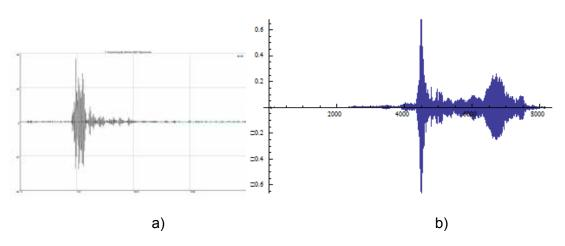
Fig. 8. a) Real signal detected by the GT200 sensor at a distance of 2 cm from a crack; b) modelled signal, which would be registered after passing 12 m along a plate with a thickness of 17 mm
