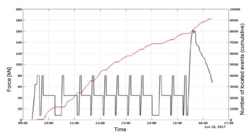
Fig. 5: Temporal course of cumulative number of localisations (red continues curve) and tensile force (black continues curve) during the test.
