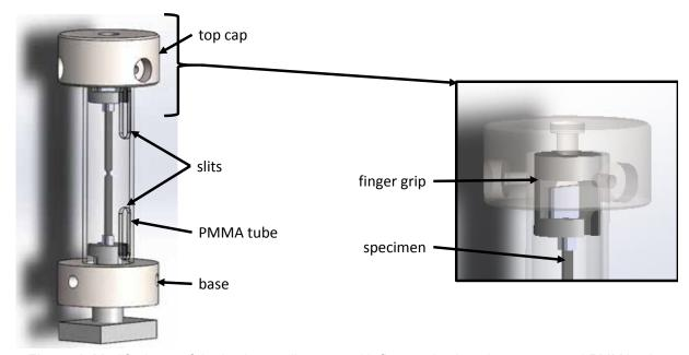
**Figure 1.** Modified part of the in situ tensile stage with finger grip clamping system and PMMA tube with two inserts for acoustic emission sensors cables.
