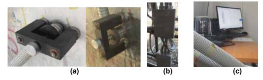
Figure 5 – (a) Sensor mounting (b) Junction box (c) Cable routing and μSamos Express-8 AE monitoring workstation
