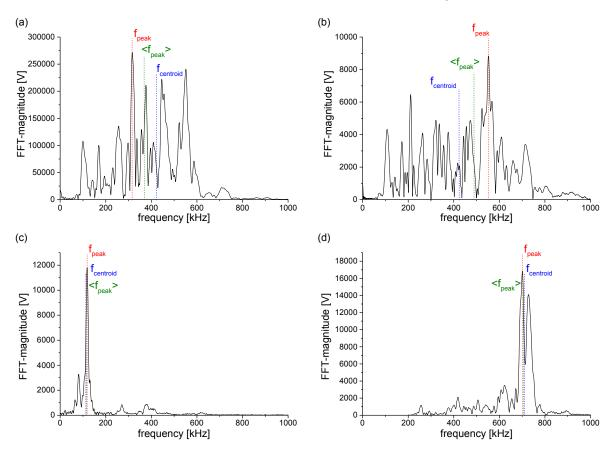
**Figure 6.** Comparison of frequency representation for four AE signals (a-d) using Peak-frequency  $f_{peak}$ , Frequency Centroid  $f_{centroid}$  and Weighted Peak-Frequency  $\langle f_{peak} \rangle$ .
