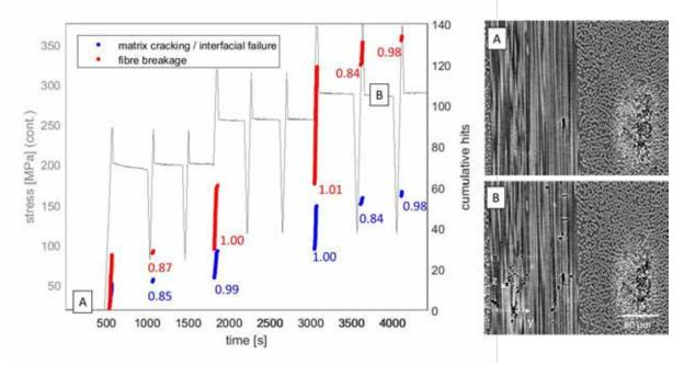
**Figure 7.** Example of layup [±45 0 ±45] including Felicity Ratios evaluated for fibre breakage signals (red) and matrix cracking / interfacial failure related signals (blue) and SRCT slices at two load levels (A-B).
