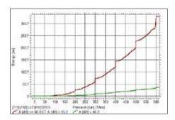
Figure 5: AE cumulative energy for medium (brown) and low (green) amplitude signals
