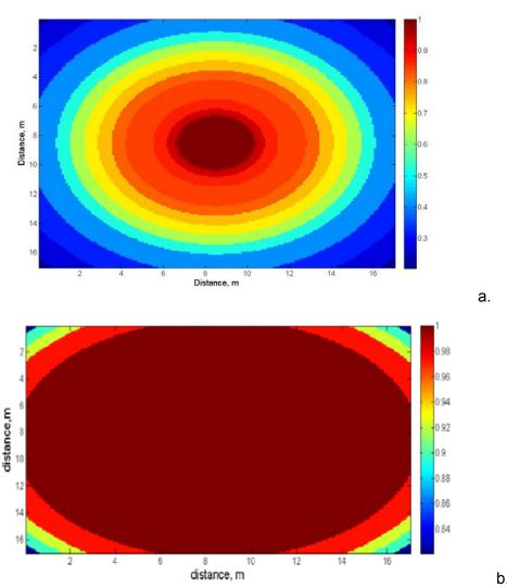
Fig.14 Two-dimensional representation of the POD diagrams (threshold level = 40 dB) a. POD for stable growing stage b. for the unstable growing stage
