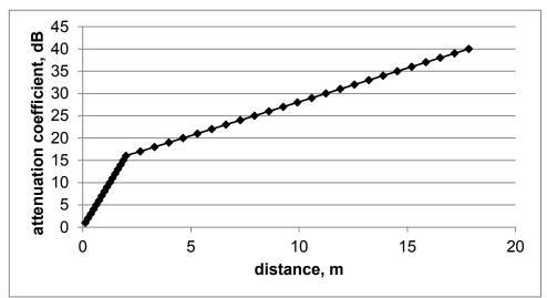
Fig.11 The attenuation coefficient depending on the distance between sensor and AE source
