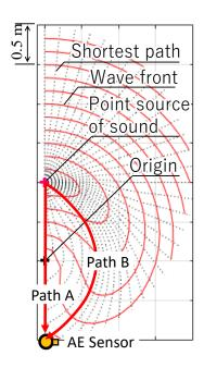
Figure 9 Shortest path for the AE in the CFRP with curved fibers [11]
