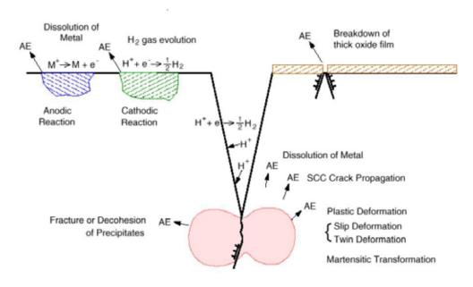
Figure 1: Sources of acoustic emission in SCC [23]
