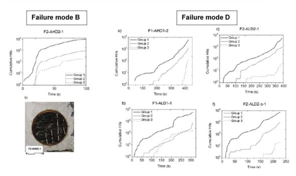
Fig. 8. Samples of CFRP fabric. Failures modes B and D. Cumulative hits against time and picture of samples.
