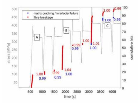
**Figure 6.** Example of layup [0 90<sub>3</sub> 0] including Felicity Ratios evaluated for fibre breakage signals (red) and matrix cracking / interfacial failure related signals (blue).
