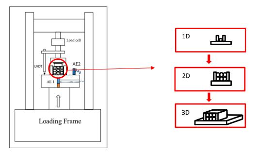
Figure 3. Diagrams of loading system for the uniaxial compression tests
