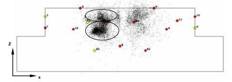
Fig. 6: Location of the 9,132 AE events in lateral view on the x-z coordinate plane.
