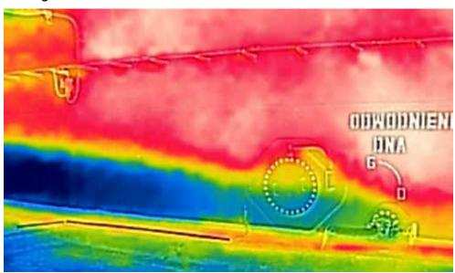
Fig 1. Thermal image of tank wall with visible sludge line
