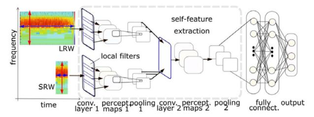
Figure 3: The structure of the CNN, where LRW and SRW denote the long rang window and short range window, respectively.
