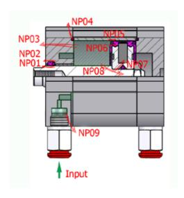
Figure 3. Leaks above the piston during retreat stroke [11]
