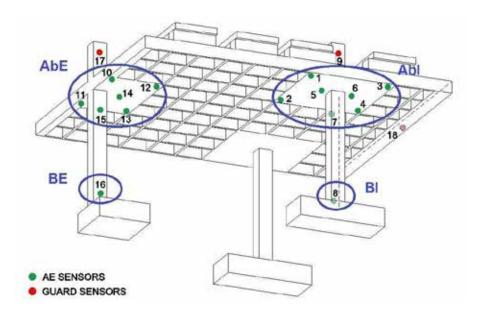
Figure 2. AE sensors layout on the specimen BS1.
