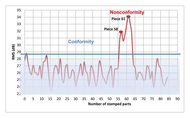
Figure 8. Evolution of RMS as function of the number of stamped parts
