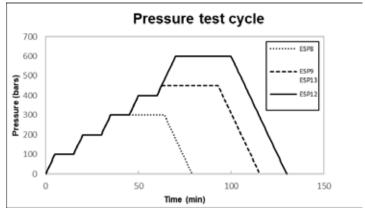
Figure 1: Pressure test cycle
