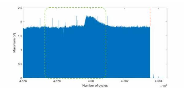
Figure 7. Maximum voltage in a burst for the last hours of the test. Area highlighted in green corresponds to an increase in the crack propagation rate. Red dashed line indicates test stopped.
