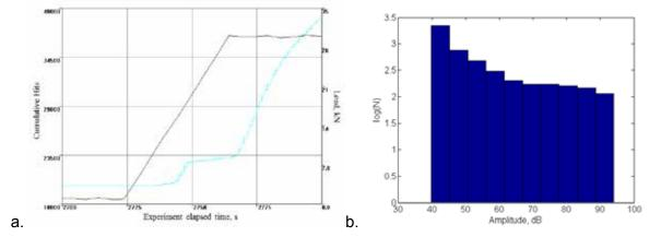
Fig. 9 – (a) Cumulative hits and the load for the RC beam, (b) Amplitude distribution for loading to 30 kN (first loading cycle of the third loading step)
