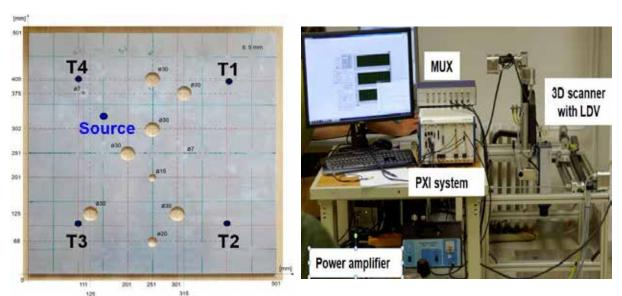
Fig.3: Left - 5 mm thin Al plate with circular holes and marked placement of four sensors T1 – T4 and Source transducer; right – experimental arrangement with scanning LDV.
