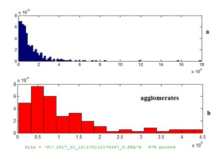
Figure 6. Burst energy distribution curves estimated within a single waveform. a) Rayleigh distribution indicating the absence of agglomerates. b)The transition to the early stage of agglomeration.
