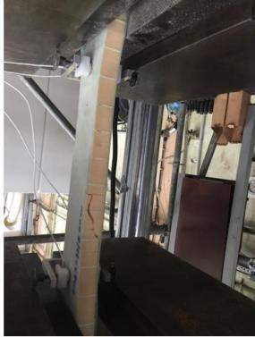
Figure 1: Tensile testing at the moment of failure - Probe CP01 [3]
