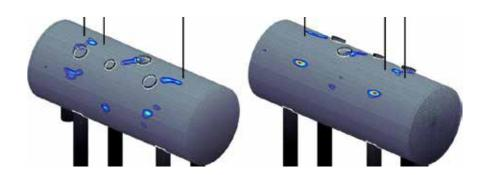
Figure 7: Kernel density estimates on the steam reservoir under IT procedure.
