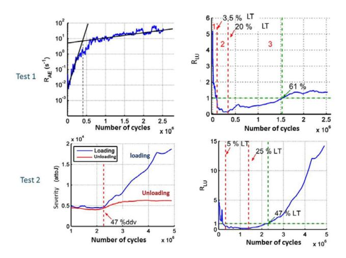
Figure 4: Evolution with the number of cycles of the coefficient  $R_{AE}$ , the coefficient  $R_{LU}$ . (LT lifetime) and the severity for two different cyclic fatigue tests at for a cyclic fatigue test at constant amplitude  $(\sigma_{max}/\sigma_r=0.36)$ .
