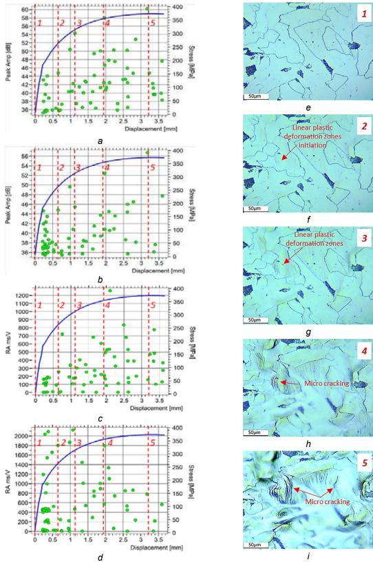
Fig. 3. Stress-strain curves of A type specimen with AE signal amplitude (a, b) and RA parameter distributions (c, d) for VS150-M type sensors (a, c) and VS75-V type sensors (c, d) as well as material microstructure images (e ÷ i) for different stress levels, magnification 400×
