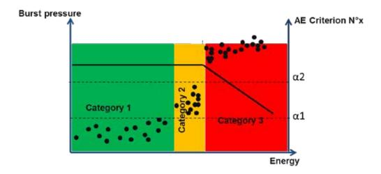
Figure 7: Burst pressure reduction curve and calibration of AE criteria protocol.
