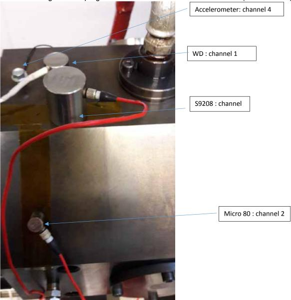
Figure 5: picture of the different sensors used for the monitoring and coupling mode.
