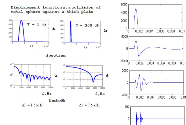
Figure 2. Displacement functions at collisions of metal spheres against a plate and the corresponding spectrums
