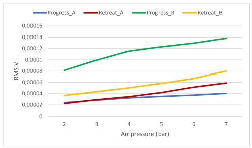
Figure 12. Effect of air pressure on the average value of RMS when sliding and pushing
