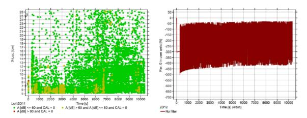
Figure 7: (left) AE linear signal source location (color-coded for AE signal amplitude) of dynamic 4-ENF tests at 5 Hz using the AE sensors on the compression side and (right) load curve for the 4-ENF specimen with the PRF adhesive.
