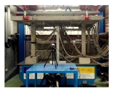
Figure 1. Experimental setup of the specimen on the shaking table.
