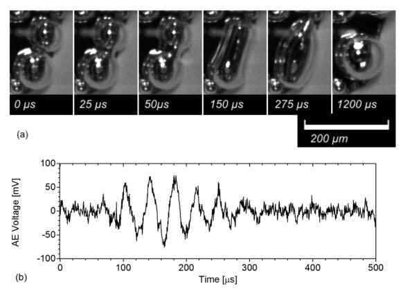
Fig. 3. Merging two hydrogen bubbles (a), and the corresponding acoustic signal (b), transducer Fujicera 1045D.
