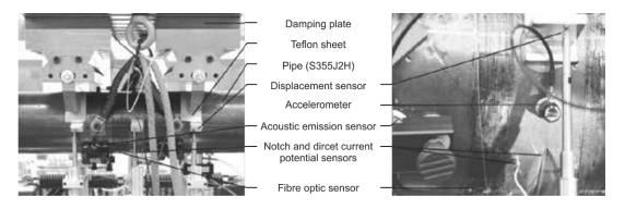
Figure 1. Experimental setup for monitoring of a four-point bending test of a 2.5 m long pipe segment by means of DCPD measurement, acoustic emission, accelerometers and fiber optical sensors.
