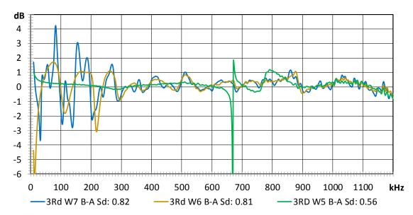
Fig. 3-6: Differences of R-sensitivity of a 150 kHz sensor, obtained by using transmitters A and B with windows signals W5 to W7.
