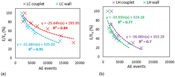
Figure 4. Stiffness modulus vs. number of AE events for (a) lime-cement masonry and (b) lime hydrate masonry.
