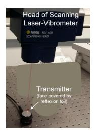
Fig. 2-4 LVM scanning the transmitter surface
