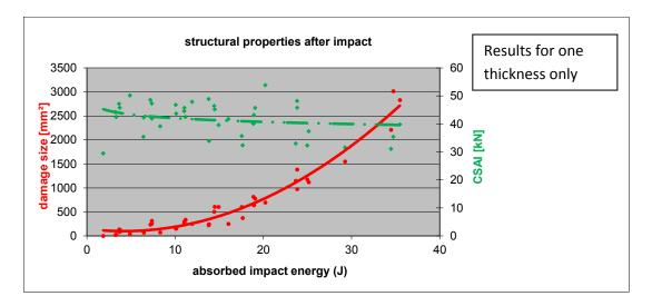
Figure 10: Compressive strength after impact and damage size over absorbed impact energy
