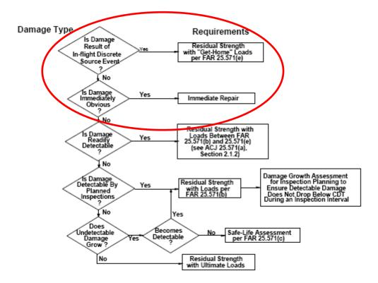
Figure 3: Levels of Damage Tolerance Assessments [4]
