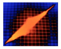
Figure 7: Lock-In-Thermography System and Screenshots with some delmainations under different Energy levels
