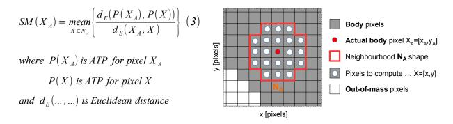
Fig.4: Definition of sensitivity parameter SM.
