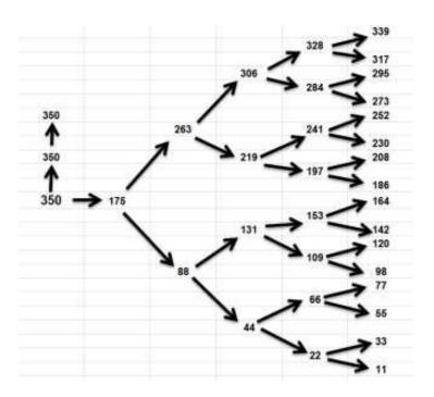
Figure 2. Experimental designs suggested by ASTM G98
