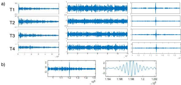
Fig 4: a). Direct burst signals of recorded 'pen-tests' by T1-T4 are plotted left, direct mixed signals under S/N = -14 dB condition are in the middle, and their TR reconstructions are right; b) Sum of reconstructions with its zoomed central part under S/N = -26 dB condition.
