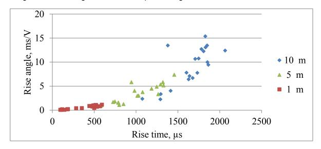
Fig.12. The scatterplot rise angle vs. rise time for the modelling signals
