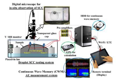
Fig. 1 Schematic of the AE measurements and SCC test incorporated with an in-situ digital microscope system.
