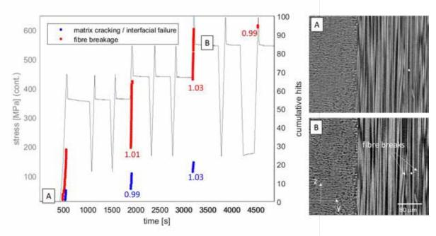
**Figure 8.** Example of layup [90 0<sub>3</sub> 90] including Felicity Ratios evaluated for fibre breakage signals (red) and matrix cracking / interfacial failure related signals (blue) and SRCT slices at two load levels (A-B).
