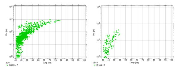
Figure 10: AE signal parameter plots (duration versus amplitude) of quasi-static tests using the broad-band AE sensor in the propagation zone of the delamination for (left) PRF and (right) HB110 adhesive (following [6]).
