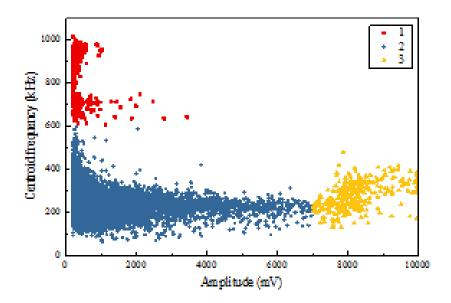
Fig. 3 Relationship between centroid frequency and amplitude of acoustic emission signal received by No. 8 sensor
