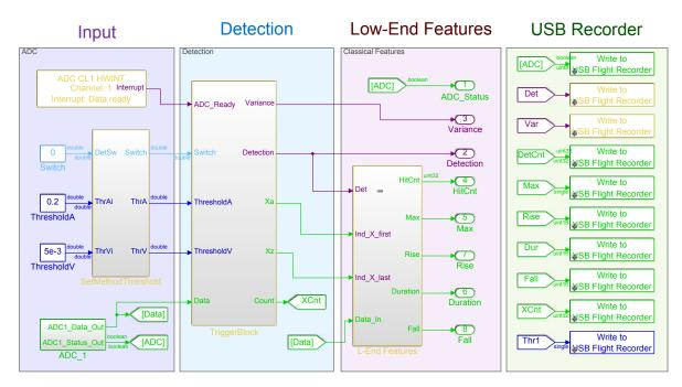
Figure 4. Simulink model of the first stages of the detection algorithm
