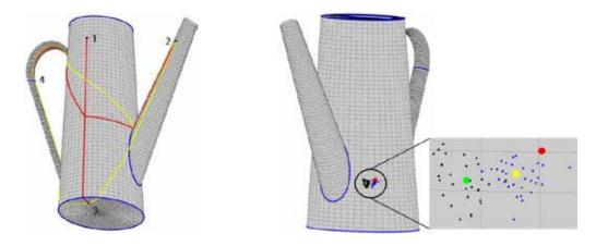
Figure 4: Sensor placement on the watering can (left) and an example of localization map using length (black+green) or time differences (blue+yellow), the source is red (right).
