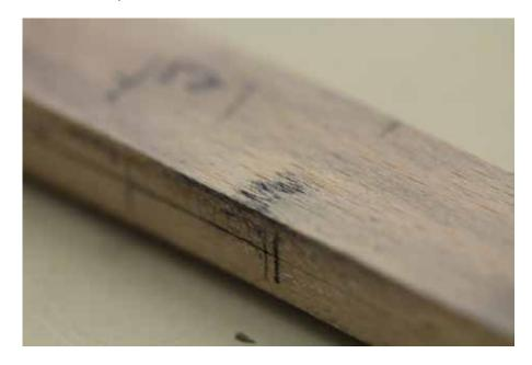
Figure 4: Photographs of the PRF-type joint showing signs of tensile failure (highlighted by black zigzag-type marks) on the bottom side after quasi-static testing, on the edge, the delamination is visible as well.
