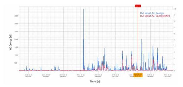
Fig. 6. AE Energy changes due to Universal Joint damage around EM Gear box
