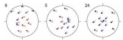
wave: blue – compression, red – dilatation. Equal-area projections of the lower focal hemisphere were applied.
