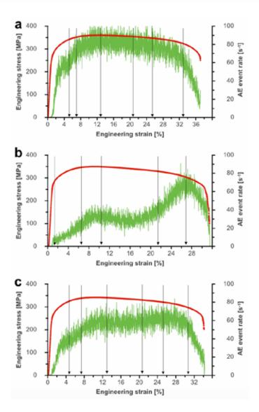
Fig. 3. Engineering stress-strain curves and corresponding acoustic emission event rate of commercially pure titanium at room temperature in a direction parallel to (a) RD (b) TD and (c) 45D. The arrows denote the strain levels at which the microstructure is investigated with EBSD.
