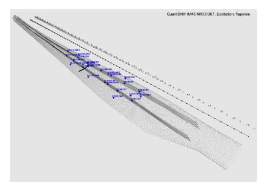
Figure 2: Spatial distribution of 24 acoustic sensors in the rotorblade
