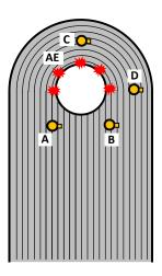
Figure 8 Suitable AE sensor locations (A and B) on CFRP with curved fibers
