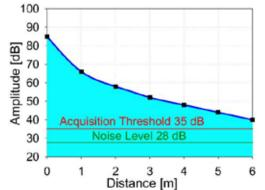
Figure 3. Experimental curve of acoustic waves damping out
