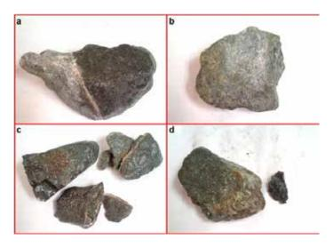
Figure 5: a) and b) Stones of the 25-31mm size category shown before discharge. c) and d) the same stones shown after discharge of 200kV and 37.5nF.
