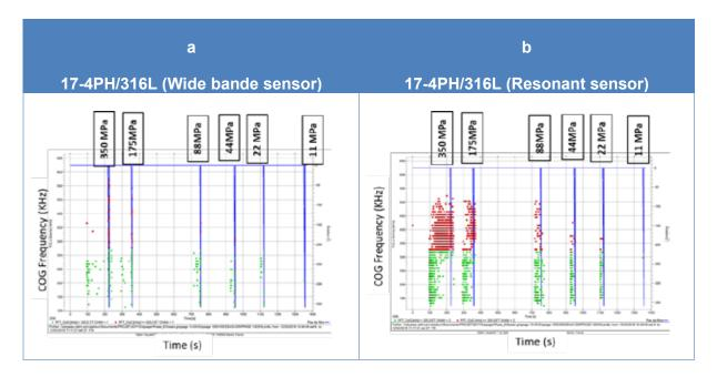
Figure 7. Distribution of the centroid frequency as function of the time test under different loads (green points represent frequency <320 KHz; red ones represent frequency >320 KHz).
