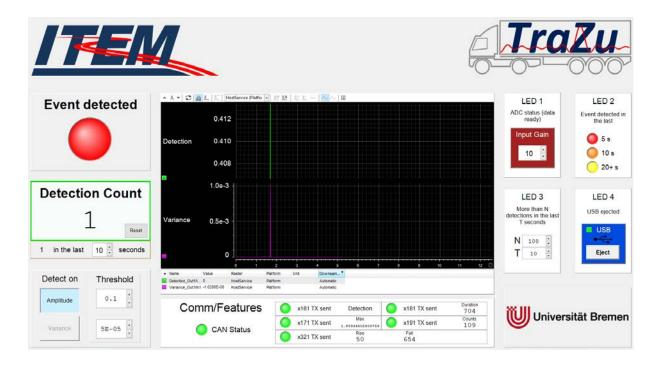
Figure 5. Graphic User Interface for the AE event detection in the MicroLabBox
