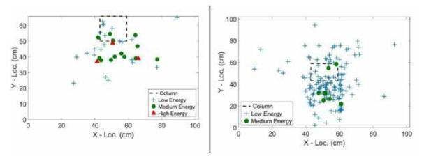
Figure 4. Localization of AE signals: Low, Medium and High Energy. AbE (left) and AbI (right).
