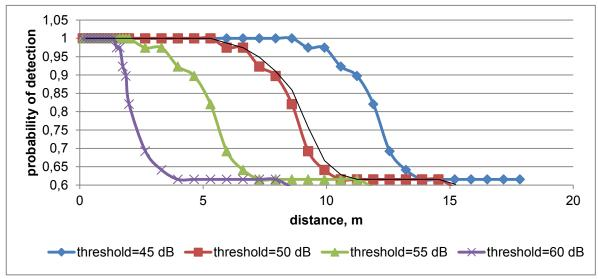
Fig.13 Probability of fatigue crack detection on the unstable growing stage depending on the distance and threshold value
