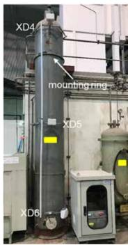
Figure 2: AET application on passivation air cylinder (urea plant)
