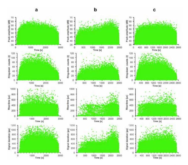
Fig. 5. Distributions of the peak amplitude, ring-down counts, signal rise-time and signal duration of the AE signals in function of time. The AE signals are received upon tensile deformation of commercially pure titanium at room temperature in a direction parallel to (a) RD (b) TD and (c) 45D.
