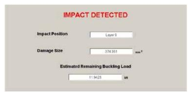
Fig. 23: Output Window for Impact Events when delamination damage is estimated based on the mean acoustic energy level and a delamination size is estimated based on the correlation of these properties. A remaining buckling load is calculated by the DDE software in this case.
