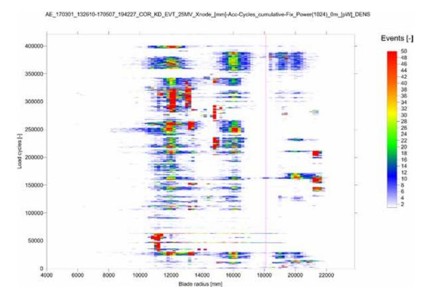
Figure 7: Events located over the radius and the load cycles
