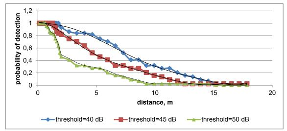
Fig.12 Probability of fatigue crack detection on the stable growing stage depending on the distance and threshold value
