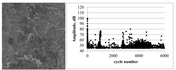
Fig. 7 a. Nonmetallic inclusions on the fractographic image; b. Dependence of AE impulse amplitudes vs. cycle number
