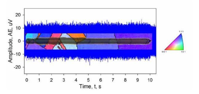
Figure 1 – Scratch test raw data, load force 1N and scratch velocity 12 mm/min: EBSD scan map of test surface superimposed with the continuous acoustic emission stream.
