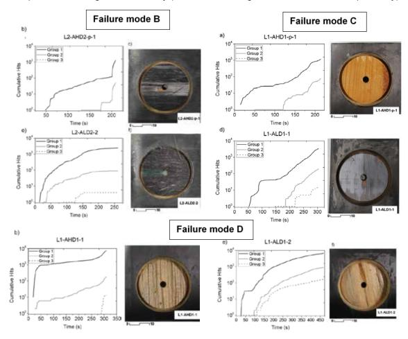
Fig. 7. Samples of CFRP laminate. Failures modes B, C and D. Cumulative hits against time and picture of samples.
