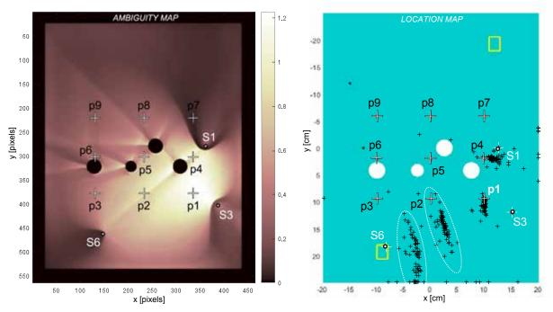
Fig.9: Location Ambiguity Map versus location results for sensor group 1-3-6.
