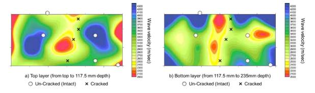
Fig. 8 Wave velocity distribution
