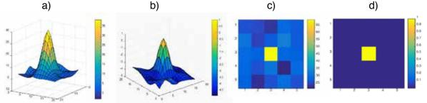
Fig. 9: 3D and flat surface mapping of resulting values detected in 5x5 mesh around the source location: a) C14 Cross Correlation Coefficients (in %), b) negative logarithms of L34 absolute lag values (both 3D pictures are 2<sup>nd</sup> order cubic interpolated), c) flat color map projections of C13 correlation coefficients without interpolation, d) L34 reciprocal time lag minima values.
