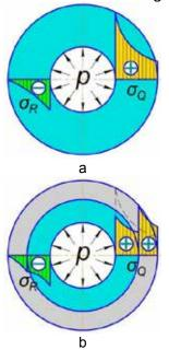
Figure 1. Stress distribution pattern in a single-walled (a) and double-walled (b) pressure vessel [1]
