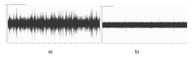
Fig.3. a) Continuous friction noise. b) AE signals from the fatigue strange experiment
