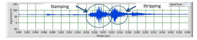
Figure 3. Acoustic emission signal of stamping + stripping
