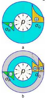
Figure 1. Stress distribution pattern in a single-walled (a) and double-walled (b) pressure vessel [1]
