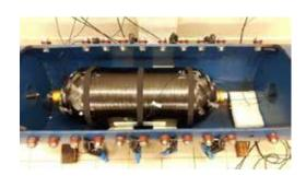
Figure 2: Distribution of the 8 used sensors on the COPV.
