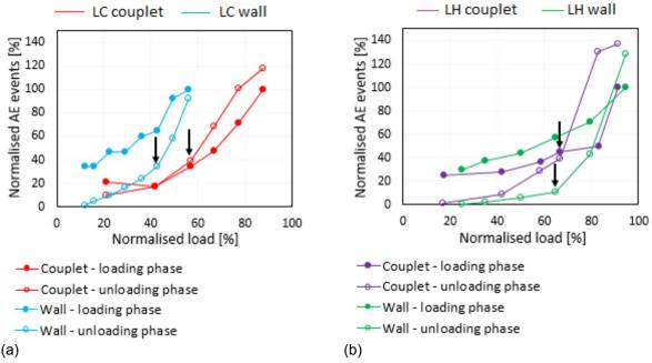
Figure 6. AE activity during loading and unloading phase for (a) lime-cement masonry and (b) lime hydrate masonry.
