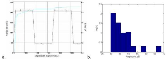
Fig. 6 – (a) Cumulative hits and the load for the RC beam, (b) Amplitude distribution for loading less than 5 kN (first loading step)
