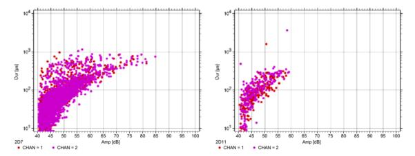
Figure 5: AE signal parameter plots (duration versus amplitude) of quasi-static tests using the AE sensors located near the starter crack tip of the 4-ENF specimens with (left) PRF and (right) HB110 adhesive (following [6]).
