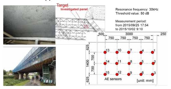
Fig. 3 Sensor arrangements for AE measurement on the real RC bridge decks
