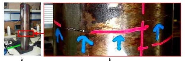
Figure 6. General view of the dismantled shell case of the reactor nozzle (a) and the increased location in the crack area (b)
