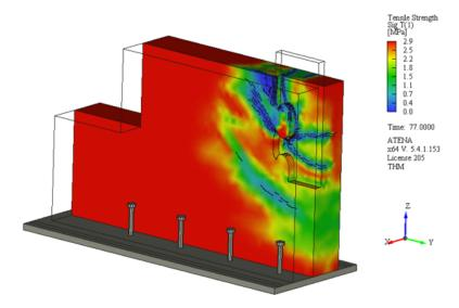
Fig. 8: Non-linear finite-element calculations of the tensile strength in projection onto a vertical cross section in the middle of the concrete dowel anchorage in a perspective view.
