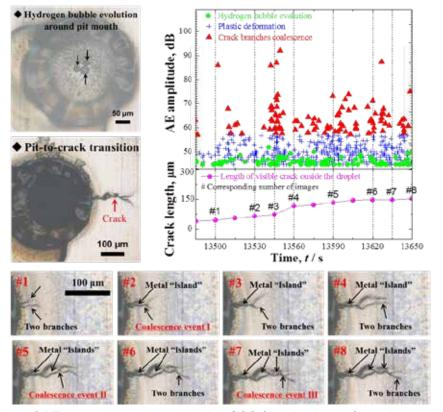
Fig. 7 Identification of AE source mechanisms during SCC from in-situ surface observation of the crack evolution (sample A).
