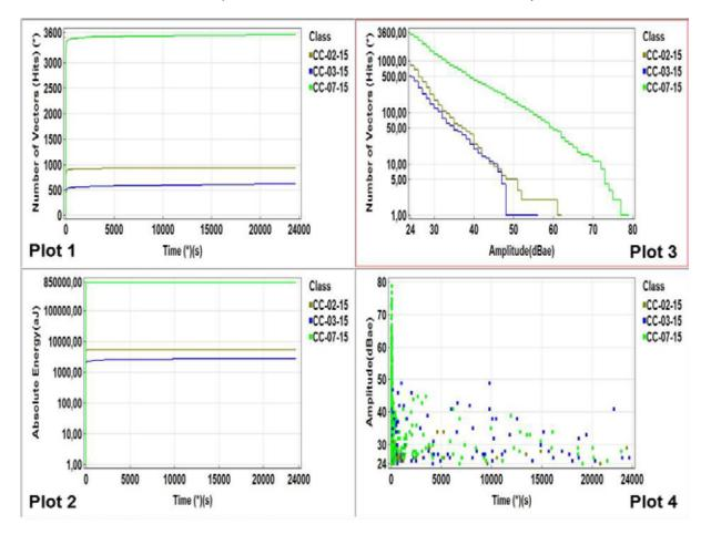
Figure 4: Filtered AE results recorded during the following tests (Stage I' [0 s - 24000 s]: CC-02-15, CC-03-15 & CC-07-15)
