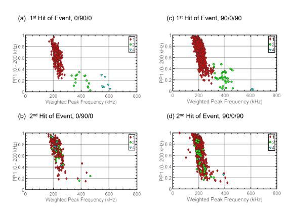
Figure 6: Signal classification through AE Features Partial Power 1 and Weighted peak frequency of 1<sup>st</sup> and 2<sup>nd</sup> Hit of events for specimen 0/90/0 (left side) and 90/0/90 (right side)
