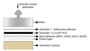
Fig. 1. Schematic representation of the materials in section.
