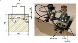
Fig. 4. Pull-off test description. Left: Schematic representation (distances in mm). Right: Image of the test. Distances in mm.
