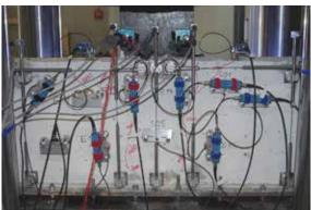
Fig. 2: Left: Perspective view of the contour of the specimen with the position of the AE sensors (red dots) and ultrasonic transmitters (yellow dots). Right: Installation situation of the specimen with the AE sensors and preamplifiers (blue boxes) and displacement sensors in vertical and axial direction.
