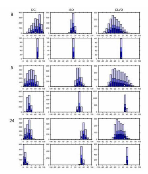
Fig. 4. Decomposition of the mechanisms for event number 9, 5 and 24. The top row in the panel corresponds to the full moment tensor (MT) solution. The bottom row corresponds to decomposition of the moment tensor corresponding to the shear-tensile crack (STC) solution. Histograms - confidence regions at the 90% (dark color), 95% (medium), and 99% (pale color) probability levels are shown.
