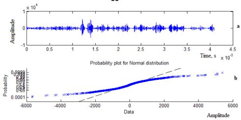
Figure 5. Waveforms characterized by disnormality: beginning of agglomeration stage
