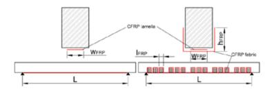
Fig. 1. LR (left) and BR (right) reinforcement layouts
