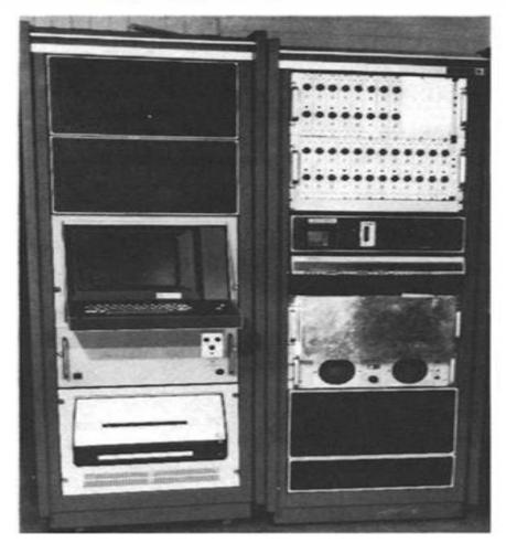
Fig 1. Westinghouse AE monitoring System, 1976
