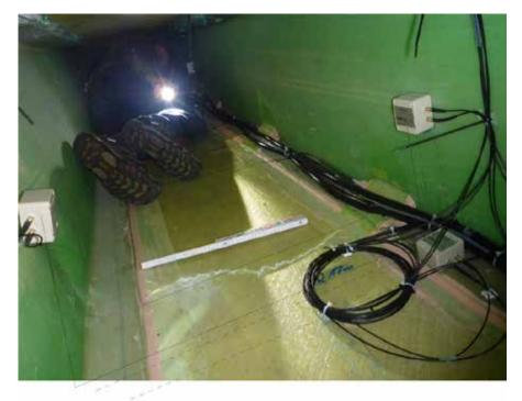
Figure 5: Medium chamber: transverse crack and failure of both spar caps at R=18,1 m
