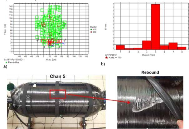
Figure 7: Vessel impacted at 3kJ@700 bar. Rejection of vessel is due to a harsh surface damage induced by the projectile rebound. A) Localization of AE sources. B) Damage induced by the rebound.
