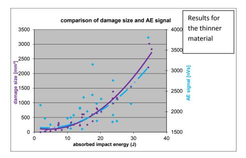
Figure 12: Comparison of damage size and AE signal over the absorbed impact energy for the thinner panThe following figure shows the correlation of damage size and the AE signal
