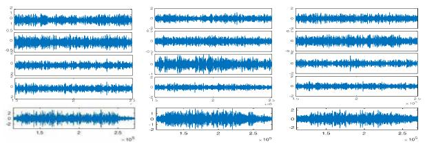
Fig.6: Comparison of TR leakage noise signals emitted by T1-T4 and reconstructed at the source position (left), at 25 mm (middle) and 50 mm (right) positions out of the source.
