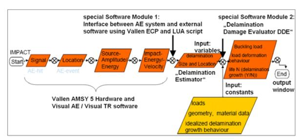
Figure 4: Flow chart of the approach for Structural Health Monitoring (SHM) of composite aerospace structures with Acoustic Emission (source: Fraunhofer LBF)
