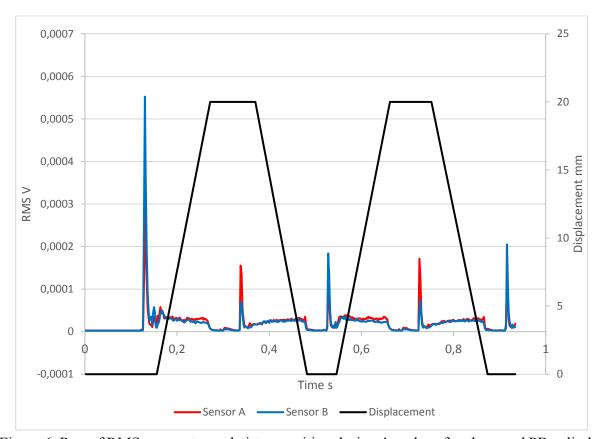
Figure 6. Run of RMS parameter and piston position during 4 cycles of undamaged PB cylinder
