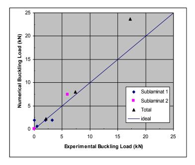
Figure 20: Buckling Loads Total and Sublaminate Buckling (source: Fraunhofer LBF)
