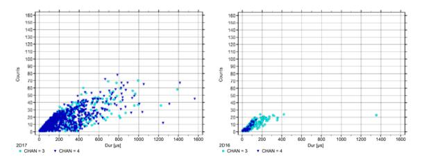
Figure 6: AE signal parameter plots (counts versus duration) of quasi-static tests using the 150 kHz resonant AE sensors located in the delamination propagation zone of the 4-ENF specimens (between the top loading rollers) for (left) PRF and (right) HB110 adhesive.
