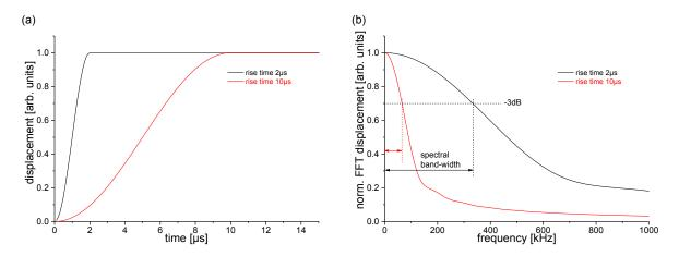
**Figure 4.** Scheme of source function (a) and corresponding spectral bandwidth estimated from -3dB drop (b).
