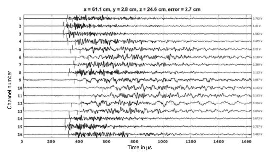
Fig. 4: Event originating from the middle of the front of specimen. The picked and calculated first (L wave) and second (T wave) arrivals are marked by vertical ticks above and below the signal traces, respectively.
