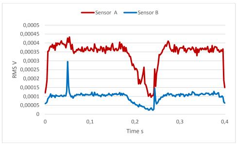
Figure 16. Damaged cylinder No.1 for one cycle
