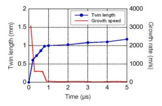
Fig.2 Evolution of length and growth speed of twin.
