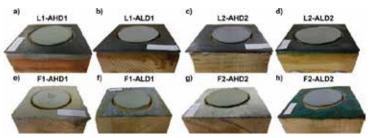
Fig. 2. Images of each type of specimen. Types of CFRP: L1: Laminate L1; L2: Laminate L2; F1: Fabric F1; F2: Fabric F2. Types of adhesives: AHD1: High density adhesive 1; ALD1: Low density adhesive 1; AHD2: High density adhesive 2; ALD2: low density adhesive 2.
