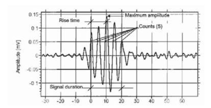
Figure 14: Possible features of acoustic signals [2]
