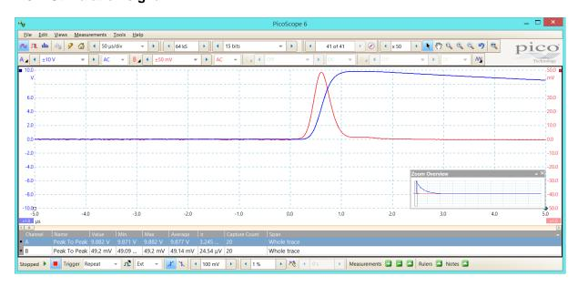
Fig. 2-5 Transmitter voltage (blue) and current (red), measured by Picoscope
