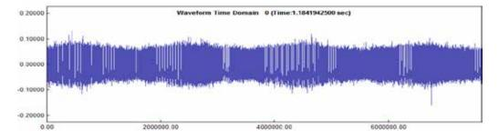
Figure 7. The pattern of the recorded noise stream (7.5 seconds) has a typical form of an amplitude modulated signal.
