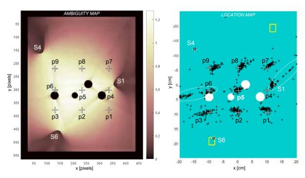
Fig.8: Location Ambiguity Map versus location results for sensor group 1-4-6.
