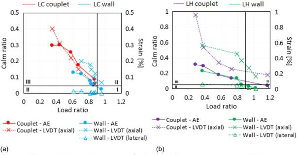
Figure 7. AE and strain-based damage quantification for (a) lime-cement masonry and (b) lime hydrate masonry.
