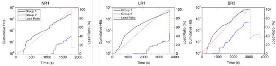
Fig. 4. Cumulative AE events versus time for an example of non-reinforced (NR), longitudinal reinforced (LR) and braided reinforced (BR) beam.
