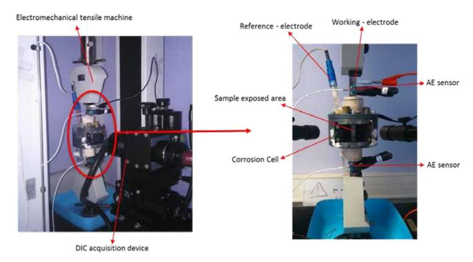
Figure 2: Experimental device used during the experiments
