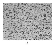
Fig. 1. The microstructure of material sections designated A (a) and B (b); magnification 500×
