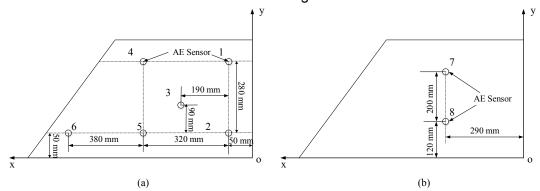
Fig. 1 Arrangement of acoustic emission sensors: (a) upper surface; (b) lower surface
