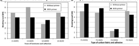
Fig. 6. Breaking load during the pull-off test for samples with CFRP. Left: Pultruded laminate.
