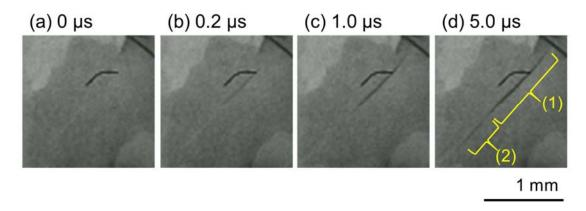
Fig. 1 Observation of twining in pure Mg by high-speed camera.
