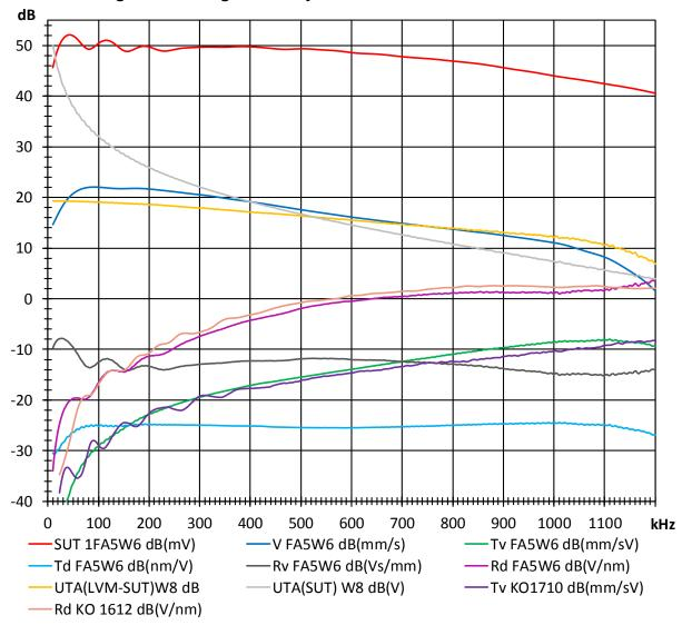
Fig. 3-4 Relevant FFT curves for sensitivity determination.
