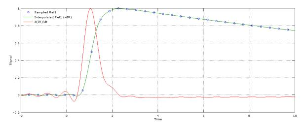
Fig. 2-6 Transmitter voltage (normalized) from LVM data (blue circles) and 40 MS/s interpolated signal (green line) and its 1<sup>st</sup> derivation du/dt (red line) that represents T-current
