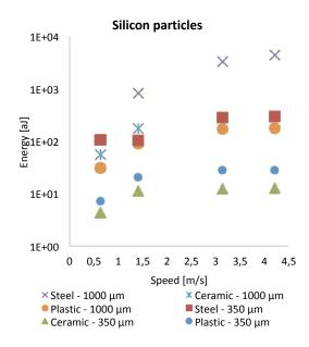
Figure 2 - Energy as function of particle's speed for silicon particles
