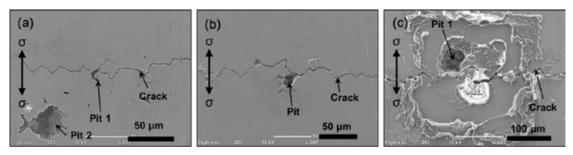
Fig. 3 SEM observations of the crack morphologies of samples (a) A, (b) B, and (c) C.
