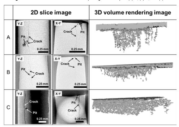
**Fig. 4** Reconstructed tomographic 2D slices and 3D volume rendering iamges of cracks morphologies of sample A, B, and C.
