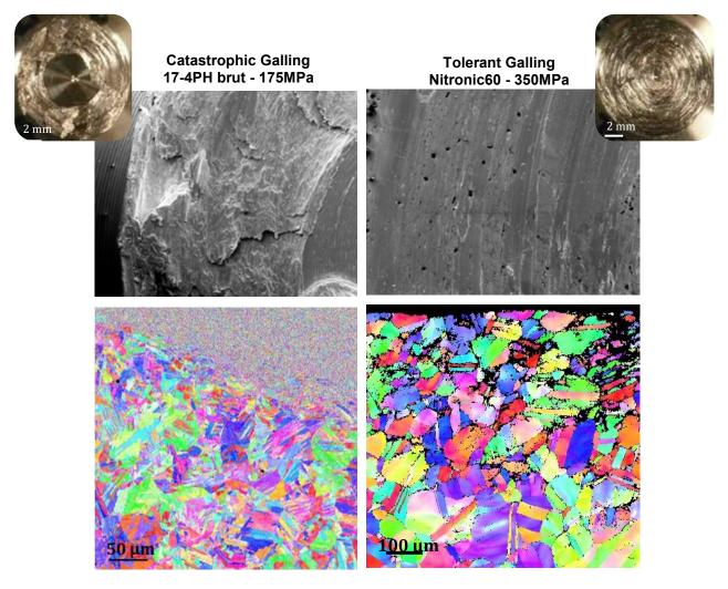
Figure 5. EBSD results (Nitronic60 (tolerant galling) and 17-4PH (catastrophic galling))
