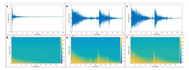
Figure 6: a) AE signal for a pulse without discharge, b) AE signal from the stone shown in Figure 2b and d, corresponding to 6% weight loss, c) Ae signal from the stone shown in Figure 2a and c, corresponding to a 44% weight loss. d), e) and f) are the corresponding sonogram.
