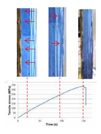
Figure 9 : Tensile test damage mecanisms Top: damage visual observation Bottom: load increase
