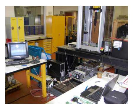
Figure 6: Overview of the test rig with the Impact Test rig in the back and the Vallen AE-system in the front
