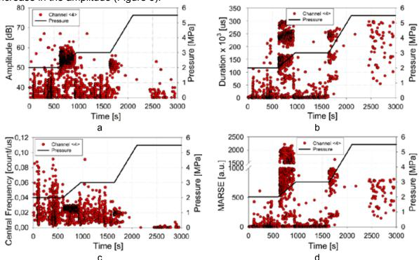
Figure 5. Graphs reflecting changes in the main assessment parameters of AE signals registered on channel 4: Amplitude (a), Duration (b), Central Frequency (c) and MARSE energy parameter (d)
