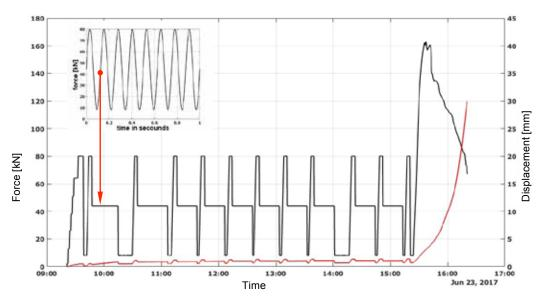
Fig. 3: Load (black continues line) and displacement behavior (red continues line) versus time. Upper left: Reduced representation of the dynamic tensile load with oscillation frequency of 8 Hz with a mean tensile force of 44 kN.
