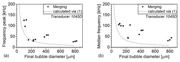
Fig. 6. (a) frequency peak and (b) median frequency of the signals collected by the transducer Fujicera 1045D.
