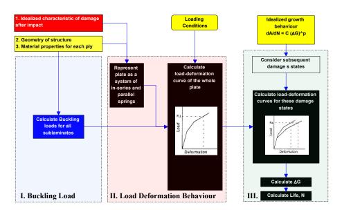
Figure 17: Schematical representation of the theoretical model that predicts damage growth (source: Fraunhofer LBF)
