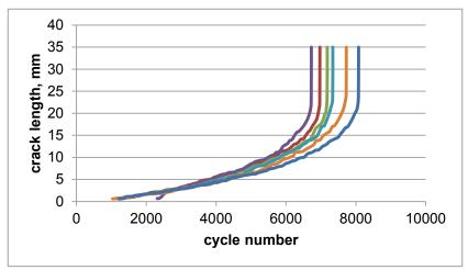
Fig. 3 Dependence of the cracks size on the number of loading cycle
