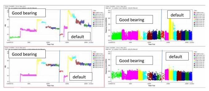
Figure 6: evolution of ASL and frequency centroid versus time with and without default. On the top graph channel 1 (WD) at the bottom channel 2 (Micro 80).
