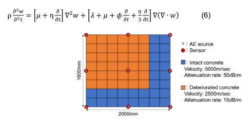
Fig. 6 Geometrical information and parametrical information for wave propagation analysis
