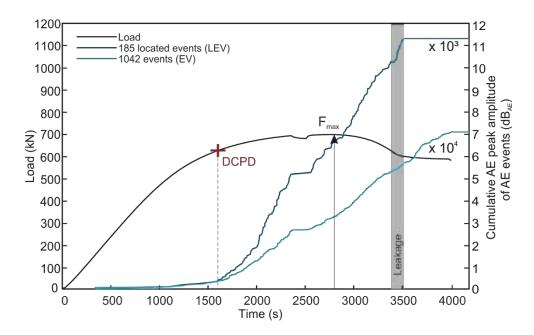
Figure 4. Load and cumulative corrected peak amplitudes of all detected AE events (1042 EV and 185 LEV) plotted vs. duration of the bending test of a pipe segment of steel. Highlighted characteristic states in the test progress are the crack initiation determined by DCPD, maximum load of 699 kN and leakage formation.
