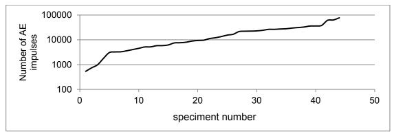
Fig.10 Number of AE impulses measured during the stable crack growth represented in the form of the ordered series
