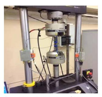
Fig. 1 The sample installed in the clamps of the testing machine
