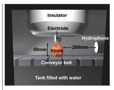
Figure 4: Schematic representation of the setup.
