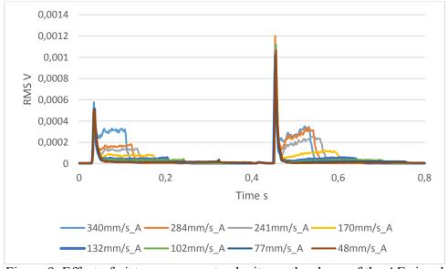
Figure 9. Effect of piston movement velocity on the shape of the AE signal
