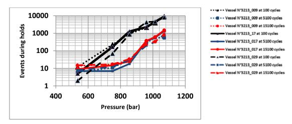
Figure 4: AE activity dispersion evaluaated for three vessels at three cycling periods.
