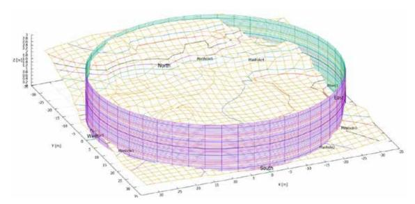
Fig 6. Spatial visualization of the sludge shape on the bottom of the tank with division into defined unit elements
