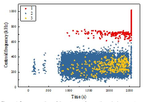
Figure 4 Occurrence time of three types of acoustic emission events
