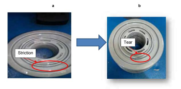
**Figure 9.** defects caused by a lack of lubrification of the tool. a. stiction which appears at fist b. Tear of the the sheet at the second time
