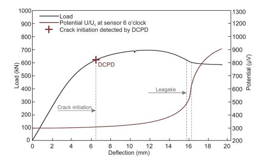
Figure 2. Load-deflection graph of the bending loaded pipe segment of steel (S355J2H). By means of the direct current potential drop (DCPD), the onset of macro cracking at the notch is detected. Leakage usually arises at the marked stage after maximum load.
